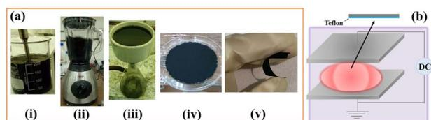
Fig. 1 Production of p-CNT-WF (a) and creation of p–n junctions across p-CNT-WF by N<sub>2</sub> plasma treatments (b). Teflon coverage is denoted by arrow.
