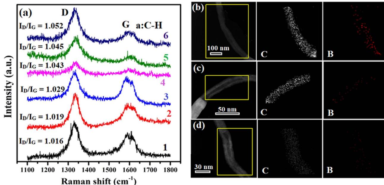
Fig. 4 Raman spectra and  $I_{\text{D}}/I_{\text{G}}$  of all samples where curve 1–6 stands for p-CNT-WF, n-CNT-WF<sub>(10min)</sub>, n-CNT-WF<sub>(20min)</sub>, B-CNT-WF, B-CNT-WF<sub>(10min)</sub> and B-CNT-WF<sub>(20min)</sub> (a). The C and B mapping on individual B-CNTs (b–d).
