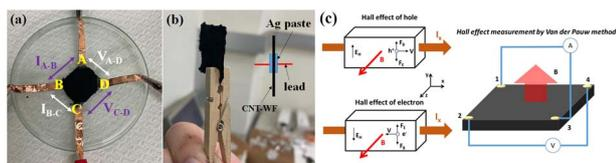
Fig. 2 Four-terminal measurements for p-CNT-WF made of different  $f_{CNT}$  (a) and two-terminal measurements for p-CNT-WF/n-CNT-WF and B-CNT-WF/n-CNT-WF (b). Schematic diagram of Hall effect (left) and the Hall effect measurement by van der Pauw method (right, c).
