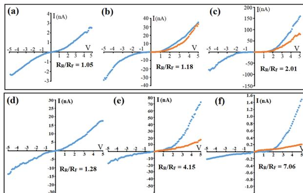
Fig. 6  $I$ - $V$  profiles of p-CNT-WF/p-CNT-WF (a), p-CNT-WF/n-CNT-WF<sub>(10min)</sub> (b), p-CNT-WF/n-CNT-WF<sub>(20min)</sub> (c), B-CNT-WF/B-CNT-WF (d), B-CNT-WF/n-CNT-WF<sub>(10min)</sub> (e) and B-CNT-WF/n-CNT-WF<sub>(20min)</sub> (f); all samples are made of  $f_{\text{CNT}} = 20$  wt%.
