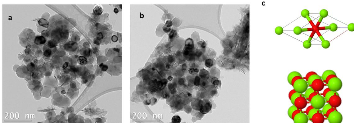
Fig. 2 (a) and (b) are TEM images of MgO nanoparticles of nominal size 50 nm. (c) Primitive cell (top) and conventional cell (bottom) of MgO nanoparticles. Green atoms are Mg<sup>2+</sup>; red atoms are O<sup>2-</sup>.
