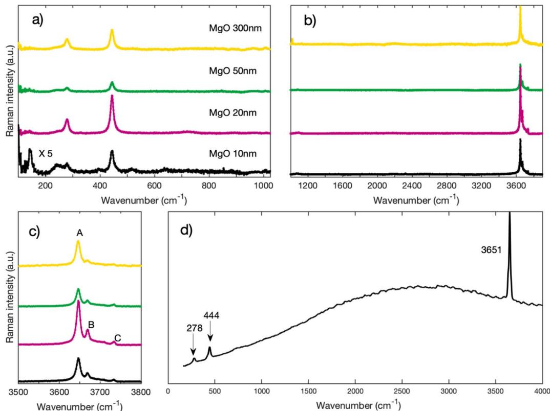
Fig. 3 (a) Raman spectra of MgO nanoparticles for low wavenumbers acquired with a grating of  $2400 \text{ l mm}^{-1}$  (b) Raman spectra of MgO nanoparticles for higher wavenumbers acquired with a grating of  $1200 \text{ l mm}^{-1}$  (c) zoom on the region around  $3700 \text{ cm}^{-1}$  of spectra of Fig. 1b. (d) Raman spectrum of  $\text{Mg}(\text{OH})_2$  from RRUFF database.<sup>31</sup>
