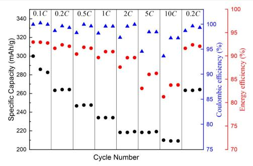
Rate capability performance of  $V_2O_5$ /SWCNT in the coin cell assembly with the lithium counter electrode cycled between 2.0 to 4.0 V.
