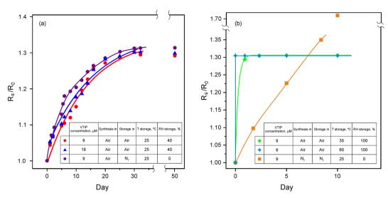
Fig. 3 Time evolution of normalized sheet resistance ( $R_0$  is the initial sheet resistance) of the  $V_2O_5$ /SWCNT composite under different conditions: (a) at 25 °C and 40% RH, (b) increased temperature and RH, and the test of VTIP/ $V_2O_5$  material.
