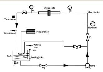
Fig. 1 Schematic diagram of the flow in the HC system.
