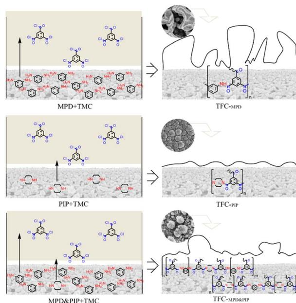
Fig. 8 Schematic of the associations between the interfacial polymerization processes using PIP and/or MPD and the structure/morphology of the TFC membranes.
