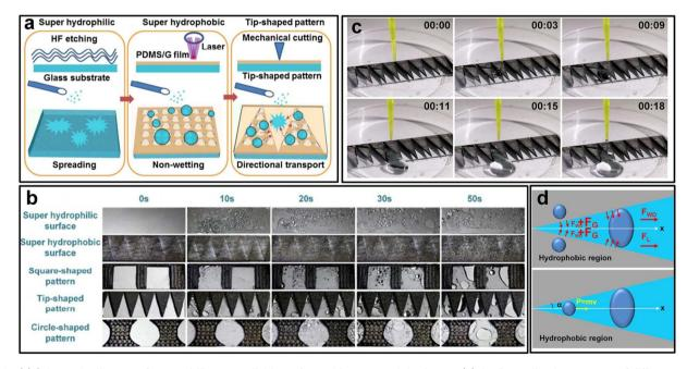
Fig. 12 (a) Schematic diagram of a wettability controllable surface with patterned tip shapes; (b) the fog collection process of different wetting surfaces; (c) directional transport of water droplets on a patterned surface with tip shapes treated at 200 °C and a 20° tip angle; (d) the water droplet was driven by the combination of Laplace pressure, gravity and wettability gradient force. 107 This figure has been adapted from ref. 107 with permission from Royal Society of Chemistry, 2018.
