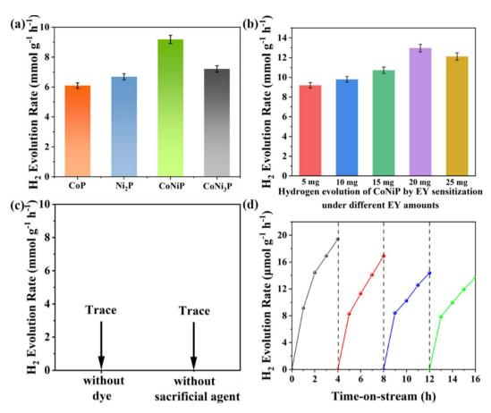
Fig. 4 (a) Photocatalytic H<sub>2</sub> evolution activities of CoP, Ni<sub>2</sub>P, CoNiP and CoNi<sub>3</sub>P with using 2.5 mg of catalysts and 5 mg of eosin-Y. (b) The photocatalytic H<sub>2</sub> evolution efficiency of CoNiP with different amount of eosin-Y. (c) The controlled experiments for testing the roles of the dye and the sacrificial agent. (d) Stability test for the CoNiP sample of H2 production (4 h for a round)
