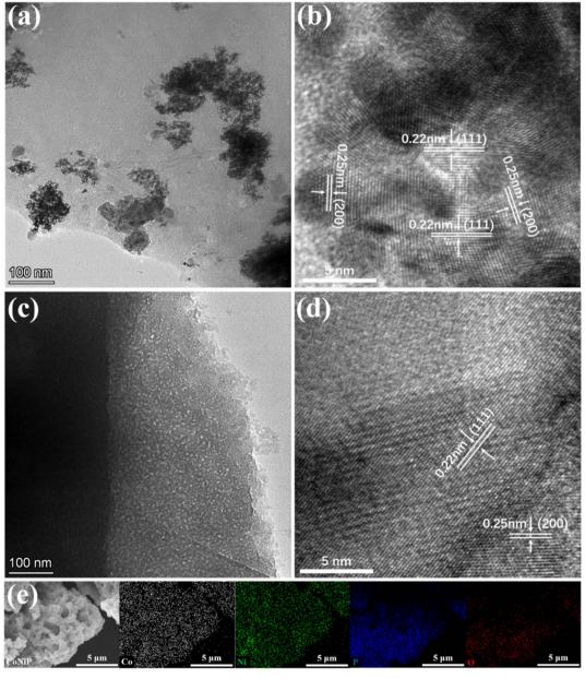
Fig. 2 The TEM and HRTEM images of (a and b) the CoNiP and (c and d) the Ni<sub>2</sub>P samples. (e) The elemental mapping images of CoNiP.
