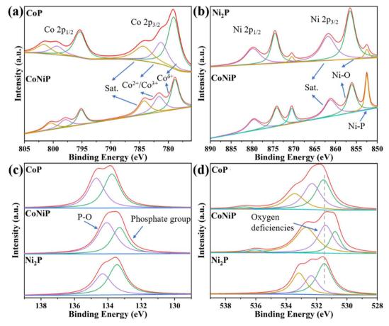
Fig. 3 The high-resolution XPS spectra of (a) Co 2p, (b) Ni 2p, (c) P 2p and (d) O 1s of CoP, CoNiP and Ni<sub>2</sub>P samples.
