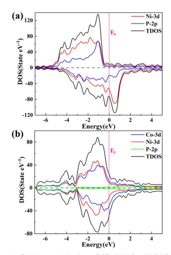
Fig. 6 Total electron density of states (DOS) of (a) Ni<sub>2</sub>P and (b) CoNiP, which projected on Co, Ni and P atoms. The Fermi level is set as zero.
