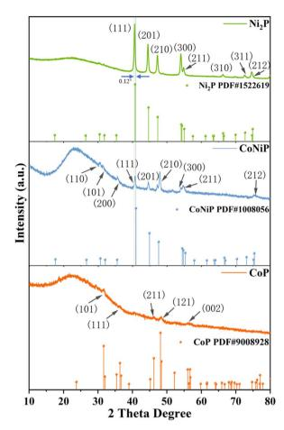
Fig. 1 Powder XRD patterns of as-prepared CoP, CoNiP and Ni<sub>2</sub>P.
