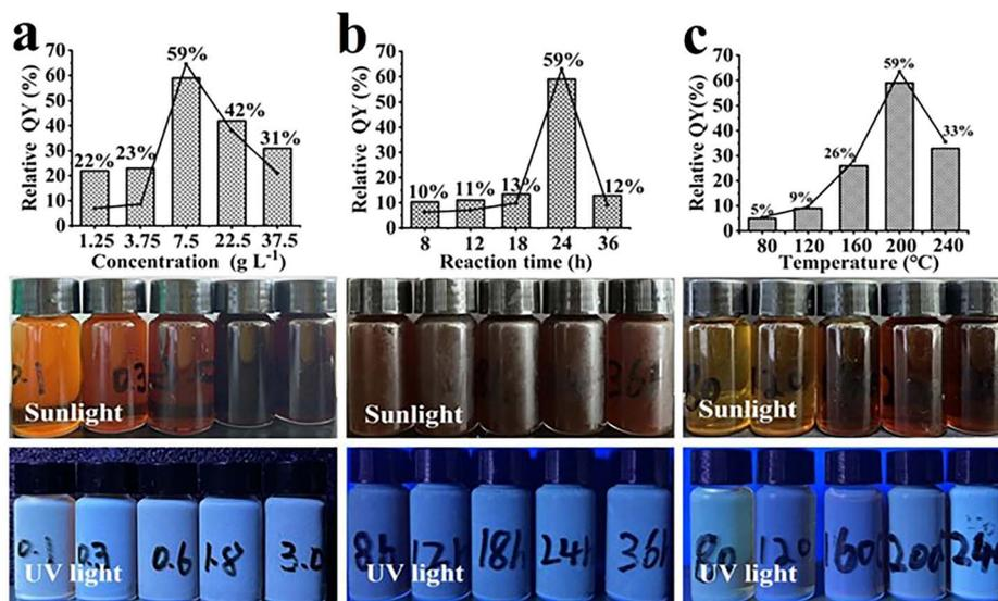
Fig. 3 Relative QY and images of CQDs under sunlight and UV irradiation under different preparation conditions. (a) Wolfberry stem concentration (1.25–37.5 g L<sup>-1</sup>), (b) reaction time (8 to 36 h), (c) temperature (80 to 240 °C).
