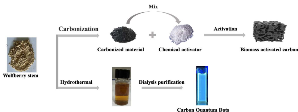
Fig. 1 Schematic preparation of CQDs and AC from wolfberry stem.
