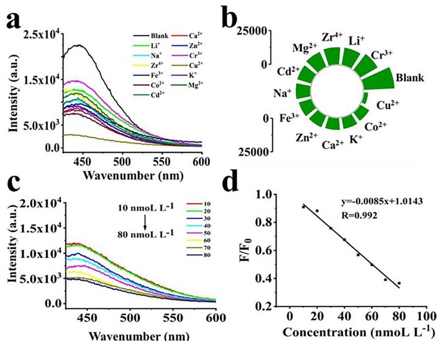
Fig. 8 (a) Fluorescence emission spectra of CQDs with 12 metal ions, (b) fluorescence intensity at 360 nm, (c) fluorescence emission spectra with different concentrations of  $\text{Cu}^{2+}$ , (d) linear curve for the detection of  $\text{Cu}^{2+}$ .
