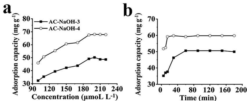
Fig. 2 (a) Isotherm adsorption and (b) dynamic adsorption of Cu<sup>2+</sup> by AC-NaOH-3 and AC-NaOH-4.
