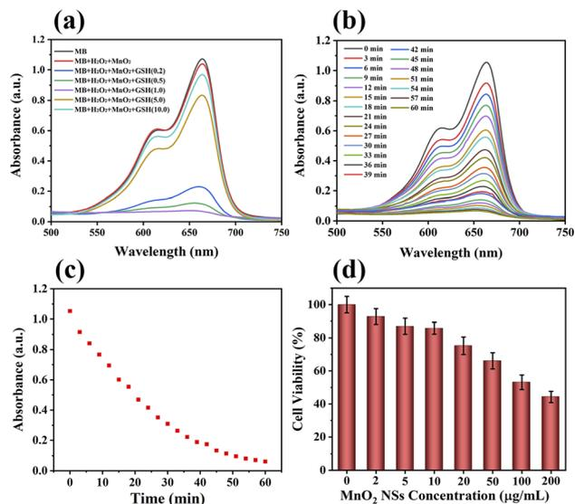
Fig. 2 (a) MB degradation by  $\text{H}_2\text{O}_2$  plus various concentrations of GSH-treated  $\text{MnO}_2$  NSs solutions (GSH: mM). (b) MB degradation after various reaction times. (c) Changes in MB degradation by  $\text{H}_2\text{O}_2$  and GSH-treated  $\text{MnO}_2$  NSs with different reaction times, measured as changes in the UV absorption intensity at 665 nm. (d) *In vitro* cytotoxicity of  $\text{MnO}_2$  NSs (0–200  $\mu\text{g mL}^{-1}$ ).
