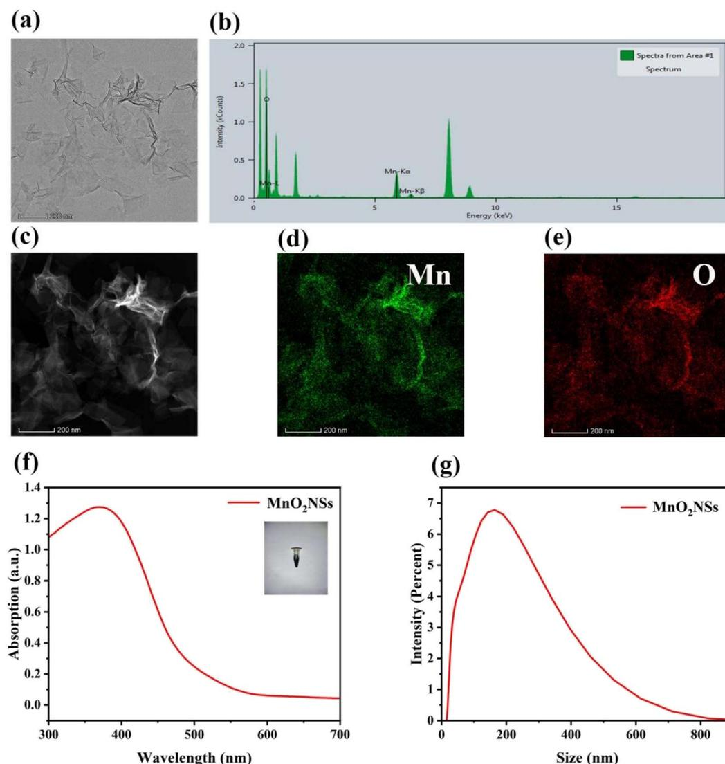
Fig. 1 (a) TEM images of MnO<sub>2</sub> NSs. (b) Energy-dispersive X-ray spectroscopy of MnO<sub>2</sub> NSs. (c–e) High-angle annular dark-field-scanning TEM images and the corresponding elemental mapping images of MnO<sub>2</sub> NSs. (f) UV spectra of MnO<sub>2</sub> NSs. (g) Size distribution of MnO<sub>2</sub> NSs.
