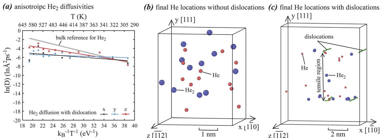
Fig. 4 Results of anisotropic diffusion of He<sub>2</sub> dimer around dislocations: (a) diffusivities, (b) final locations of He and He<sub>2</sub> collected from the 26 diffusion simulations for the dislocation-free systems, and (c) final locations of He and He<sub>2</sub> collected from the 26 diffusion simulations for the dislocation-containing systems.
