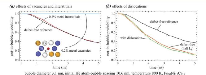
Fig. 5 Time distribution for the diffusion He atom not to join the bubble as a function of time: (a) effects of vacancies and interstitials, and (b) effects of dislocations.
