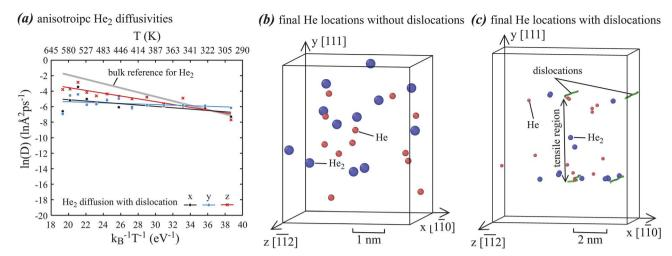
Fig. 4 Results of anisotropic diffusion of  $He_2$  dimer around dislocations: (a) diffusivities, (b) final locations of He and  $He_2$  collected from the 26 diffusion simulations for the dislocation-free systems, and (c) final locations of He and  $He_2$  collected from the 26 diffusion simulations for the dislocation-containing systems.
