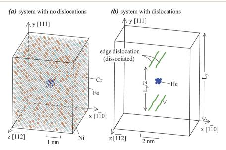
Fig. 1 Crystal geometries used for He cluster diffusion simulations: (a) systems without dislocations (white balls: Fe, blue balls: Ni, orange balls: Cr), and (b) systems with dislocations.
