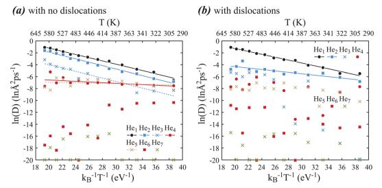
Fig. 3 Logarithm of MD diffusivities for He clusters with sizes 1–7 as a function of  $(k_B T)^{-1}$   $(k_B$  is Boltzmann constant and T is temperature): (a) systems with no dislocations, and (b) systems with dislocations.
