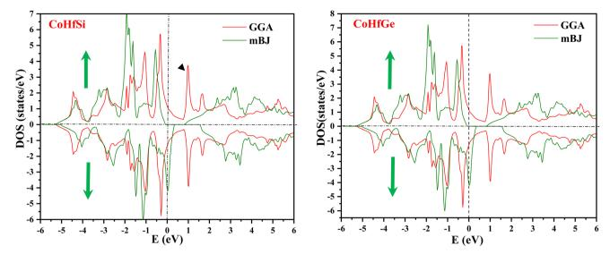
Fig. 7 Calculated total density of states for CoHfSi and CoHfGe by GGA and mBJ
