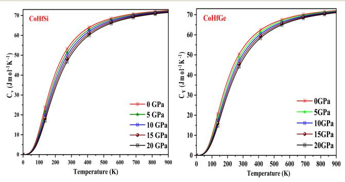
Fig. 14 The variation of specific heat with the temperature at different pressure of CoHfSi and CoHfGe half Heusler alloys.
