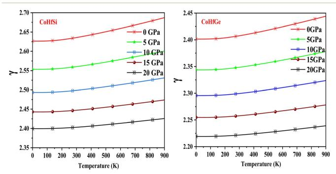
Fig. 16 The variation of the Grüneisen parameter with the temperature at different the pressure of CoHfSi and CoHfGe half Heusler alloys.
