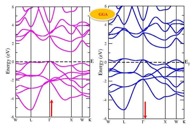
Fig. 4 Spin polarised band structure of CoHfGe alloy via GGA method.
