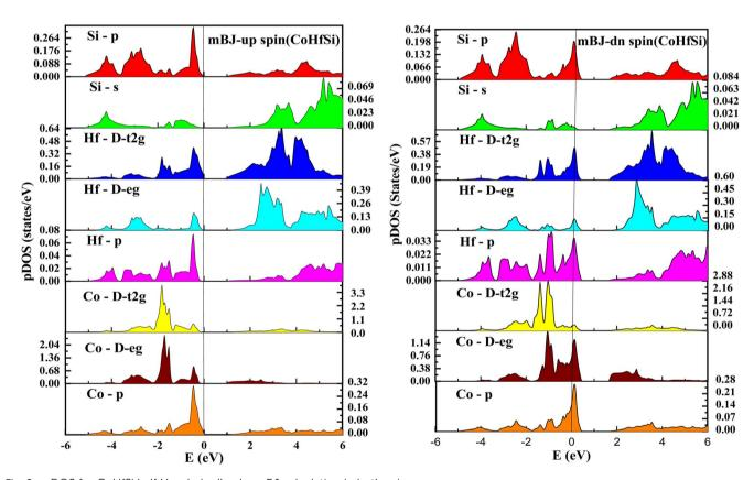
Fig. 8 pDOS for CoHfSi half Heusler's alloy by mBJ calculation in both spins.
