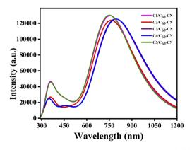
Fig. 10 Plot of absorption spectra of the studied C1-C5/C<sub>60</sub>-CN complexes.
