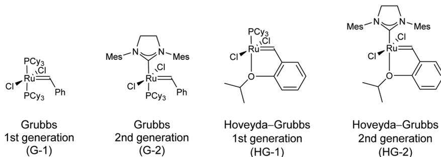
Fig. 1 The most commonly used commercially available Ru-based metathesis catalysts. Cy = cyclohexyl, Mes = 2,4,6-trimethylphenyl.
