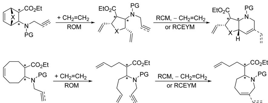
**Scheme 4** Earlier work: synthesis of azaheterocyclic  $\beta$ -amino esters *via* ring-rearrangement metathesis. X = O, CH<sub>2</sub>. PG = Boc, Ts.
