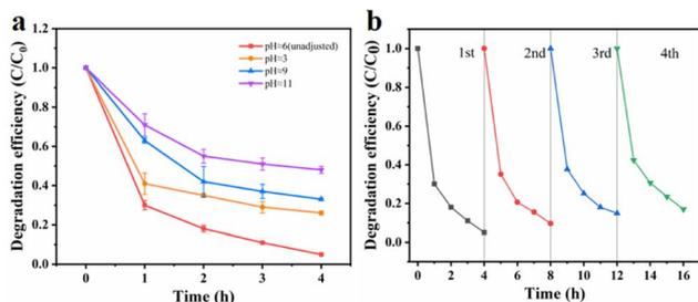
Fig. 6 Effect of reaction parameters on TCE degradation: initial pH value (a) and reusability of  $\text{MnCo}_2\text{O}_4/\text{rGO}$  as a catalyst activated PS for the degradation of TCE (b) [reaction conditions: PS dosage =  $0.3 \text{ g L}^{-1}$ , catalyst dosage =  $0.3 \text{ g L}^{-1}$  and reaction temperature =  $25 \text{ }^\circ\text{C}$ ].
