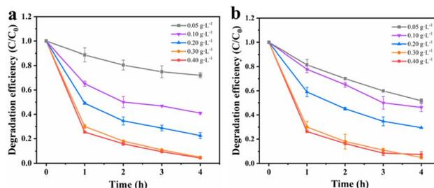
Fig. 5 Effect of reaction parameters on TCE degradation: (a) catalyst dosage [PS dosage =  $0.3 \text{ g L}^{-1}$ ] and (b) PS dosage [catalyst dosage =  $0.3 \text{ g L}^{-1}$ ] [reaction conditions: reaction temperature =  $25 \text{ }^\circ\text{C}$  and initial pH value = 6 (unadjusted)].
