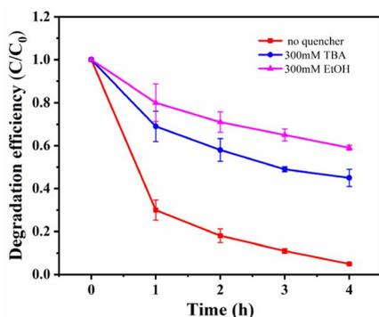
Fig. 8 Effects of different radical quencher for the TCE degradation in  $\text{MnCo}_2\text{O}_4/\text{rGO}/\text{PS}$  system [reaction conditions: PS dosage =  $0.3 \text{ g L}^{-1}$ , catalyst dosage =  $0.3 \text{ g L}^{-1}$ , reaction temperature =  $25^\circ\text{C}$  and initial pH value = 6 (unadjusted)].
