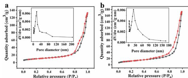
Fig. 3 Nitrogen adsorption–desorption isotherm plots of (a)  $\text{MnCo}_2\text{O}_4$  and (b)  $\text{MnCo}_2\text{O}_4/\text{rGO}$  and BJH pore distribution (inset).
