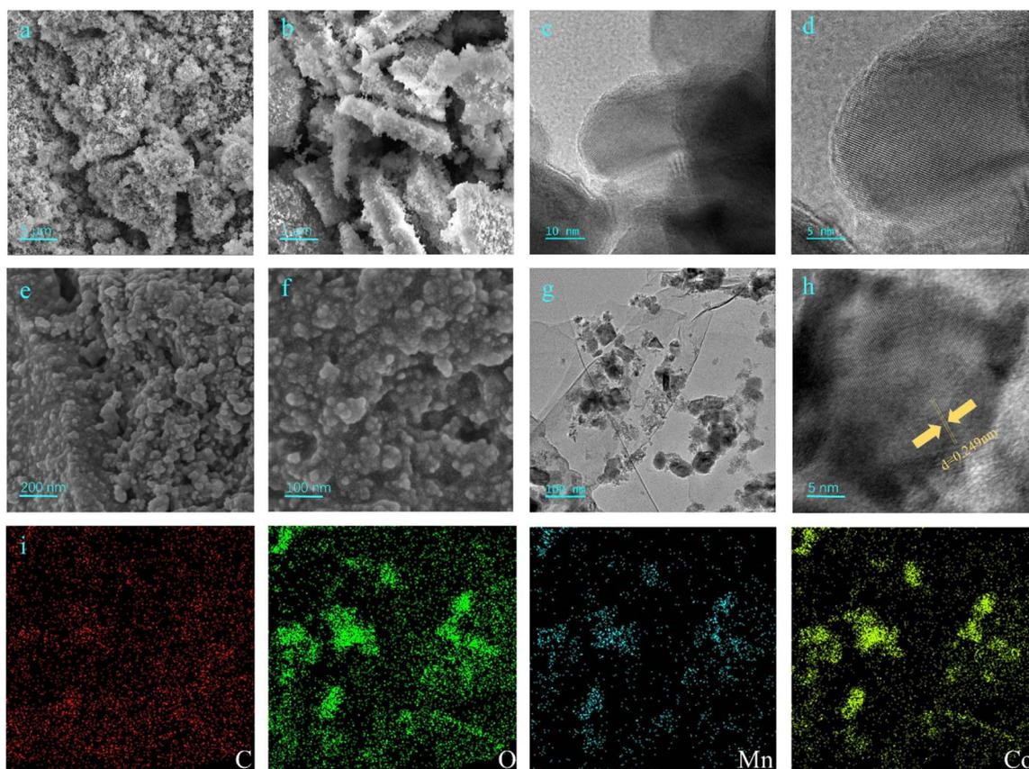
Fig. 2 SEM (a) and (b), TEM (c) and HRTEM (d) images of  $\text{MnCo}_2\text{O}_4$  nanoparticle, SEM (e) and (f), TEM (g), HRTEM (h) and STEM-EDX (i) images of the as-synthesized  $\text{MnCo}_2\text{O}_4/\text{rGO}$  nanocomposite.
