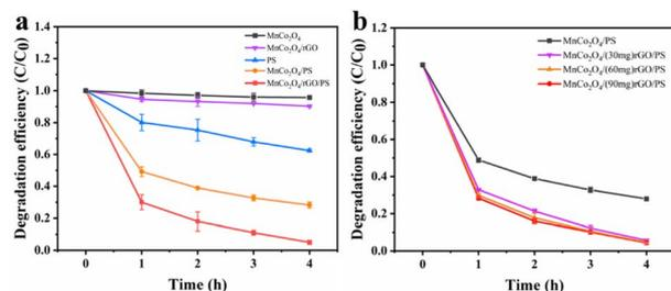
Fig. 4 Degradation efficiency of TCE in different systems (a) and effect of rGO loading on TCE degradation (b) [reaction conditions: persulfate concentration =  $0.3 \text{ g L}^{-1}$ , catalyst dosage =  $0.3 \text{ g L}^{-1}$ , reaction temperature =  $25 \text{ }^\circ\text{C}$  and initial pH value = 6 (unadjusted)].
