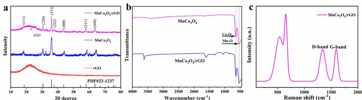
Fig. 1 (a) XRD patterns of the as-synthesized rGO,  $\text{MnCo}_2\text{O}_4$  and  $\text{MnCo}_2\text{O}_4/\text{rGO}$  samples; (b) FT-IR spectroscopy of  $\text{MnCo}_2\text{O}_4$  and  $\text{MnCo}_2\text{O}_4/\text{rGO}$  samples; (c) Raman spectroscopy of  $\text{MnCo}_2\text{O}_4/\text{rGO}$  sample.
