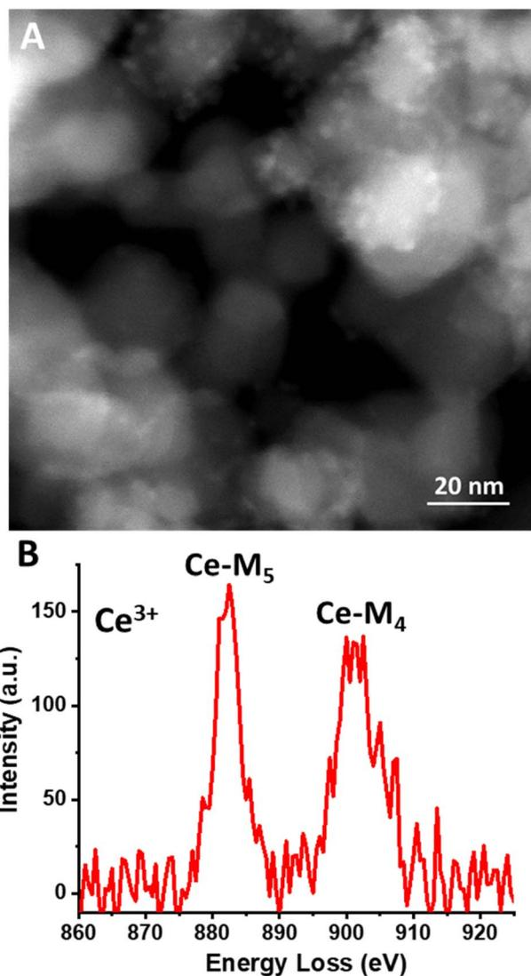
Fig. 7 (A) HAADF-STEM image of Ce-carbonate deposited onto TiO<sub>2</sub> that was thoroughly washed with pH 6 aqueous solution and exhibits Ce(III) carbonate clusters ( $\approx 2.5$  nm) deposited on the TiO<sub>2</sub> surface with no evidence of changes in morphology or degradation as a result of the wash. (B) Cerium electron energy loss spectrum (EELS) of Ce-carbonate cluster deposited onto TiO<sub>2</sub> that was thoroughly washed with pH 6 aqueous solution in (A).
