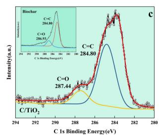
Fig. 9 XPS spectra of C/TiO<sub>2</sub> (a), Ti 2p in C/TiO<sub>2</sub> and biochar (b), and C 1s in C/TiO<sub>2</sub> and biochar (c).
