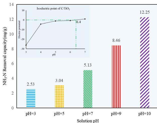
Fig. 5 NH<sub>3</sub>-N removal capacity at different initial solution pH values (AM1.5, 25 A, 1 g L<sup>-1</sup> C/TiO<sub>2</sub>, C<sub>0</sub> = 50 mg L<sup>-1</sup>).
