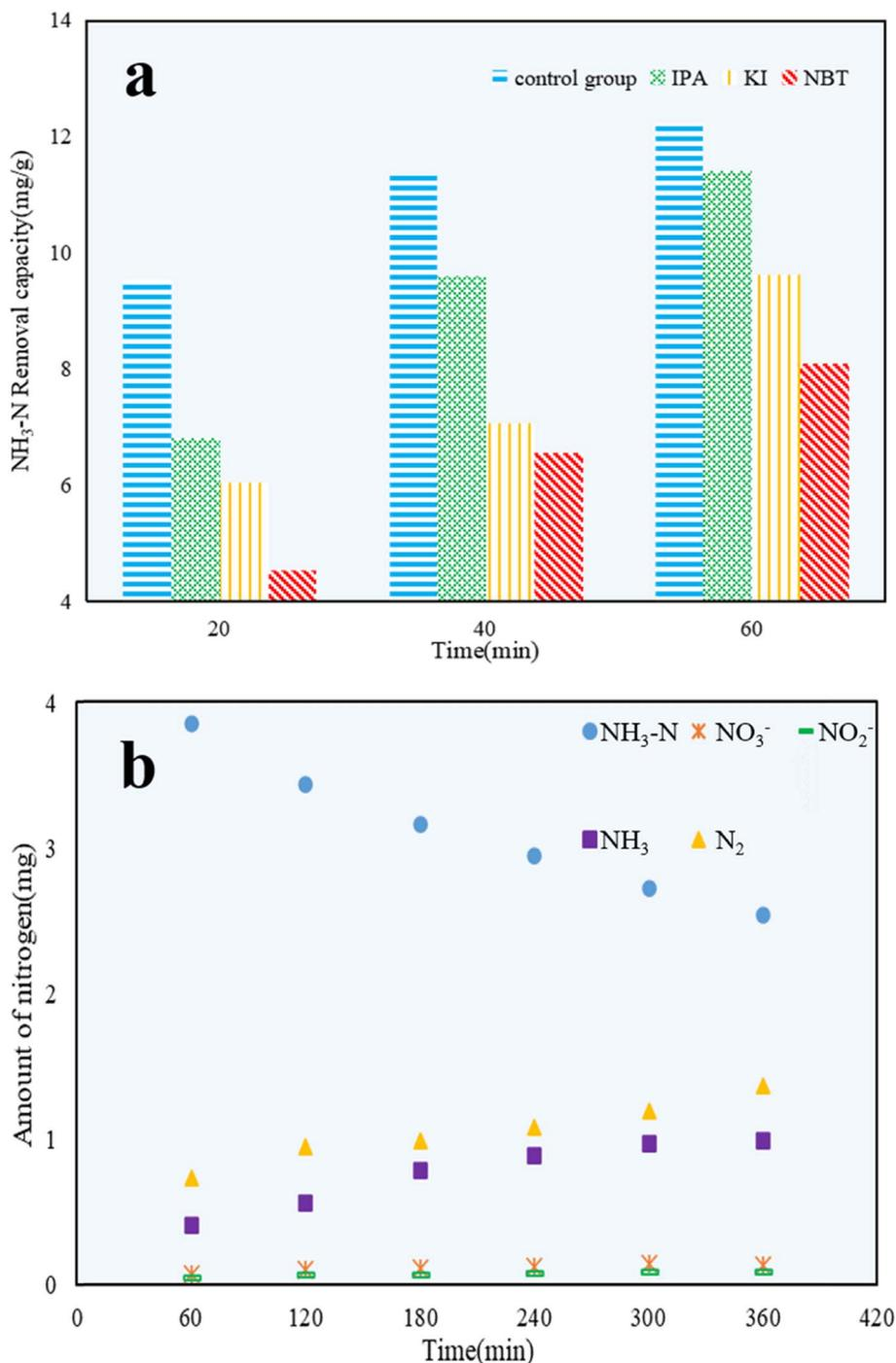
Fig. 11  $\text{NH}_3\text{-N}$  removal capacity under different quenching agents (a), and plot of the amounts of  $\text{NH}_3\text{-N}$ ,  $\text{NO}_3^-$ ,  $\text{NO}_2^-$ ,  $\text{NH}_3$ , and  $\text{N}_2$  in the reaction system (b) ( $\text{AM}1.5$ , 25 A,  $1 \text{ g L}^{-1} \text{ C}/\text{TiO}_2$ , pH 10.0,  $C_0 = 50 \text{ mg L}^{-1}$ ).
