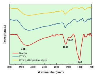
Fig. 10 FT-IR spectra of C/TiO<sub>2</sub> and biochar.
