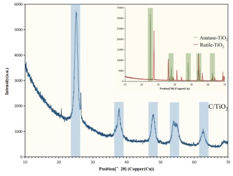
Fig. 8 XRD spectra for C/TiO<sub>2</sub>, anatase-TiO<sub>2</sub>, and rutile-TiO<sub>2</sub>.
