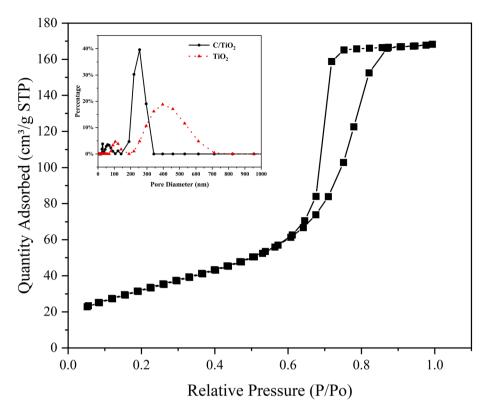
Fig. 7 N<sub>2</sub> adsorption/desorption isotherms of C/TiO<sub>2</sub> and the pore-size distribution curves of TiO<sub>2</sub> and C/TiO<sub>2</sub>.
