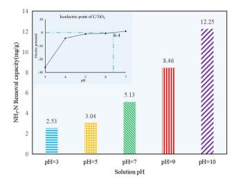
Fig. 5 NH<sub>3</sub>–N removal capacity at different initial solution pH values (AM1.5, 25 A, 1 g  $L^{-1}$  C/TiO<sub>2</sub>,  $C_0 = 50$  mg  $L^{-1}$ ).
