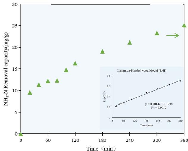
Fig. 3  $\text{NH}_3\text{-N}$  removal capacity at different irradiation times by the  $\text{C}/\text{TiO}_2$  photocatalysts (AM1.5, 25 A,  $1 \text{ g L}^{-1} \text{ C}/\text{TiO}_2$ , pH 10.0,  $C_0 = 50 \text{ mg L}^{-1}$ ).
