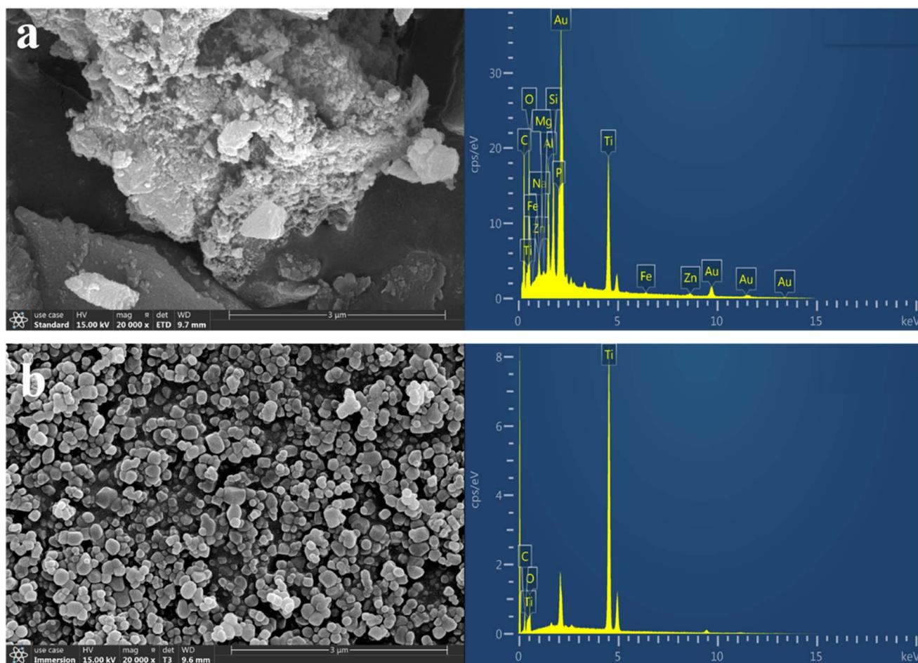
Fig. 6 SEM-EDS analysis for C/TiO<sub>2</sub> and TiO<sub>2</sub> (a) C/TiO<sub>2</sub>; (b) TiO<sub>2</sub>.
