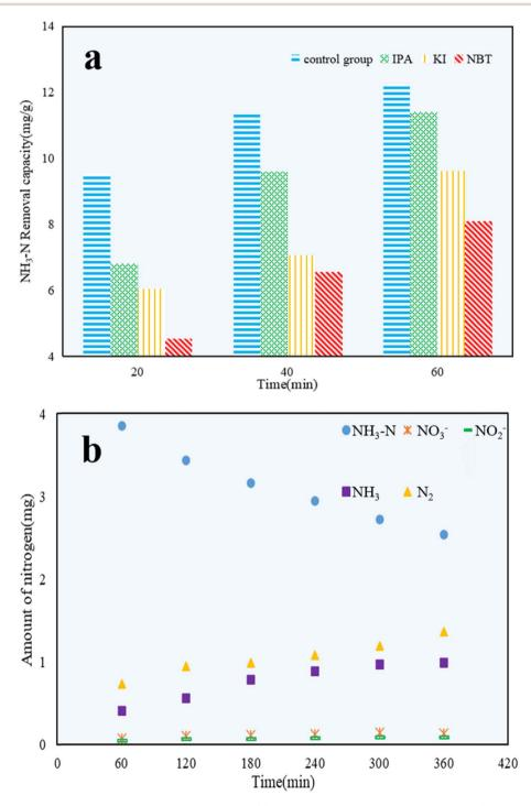
Fig. 11 NH<sub>3</sub>-N removal capacity under different quenching agents (a), and plot of the amounts of NH<sub>3</sub>-N, NO<sub>3</sub><sup>-</sup>, NO<sub>2</sub><sup>-</sup>, NH<sub>3</sub>, and N<sub>2</sub> in the reaction system (b) (AM1.5, 25 A, 1 g L<sup>-1</sup> C/TiO<sub>2</sub>, pH 10.0,  $C_0 = 50$  mg L<sup>-1</sup>).
