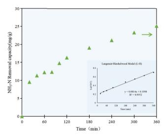
Fig. 3  $\,$  NH<sub>3</sub>-N removal capacity at different irradiation times by the C/TiO<sub>2</sub> photocatalysts (AM1.5, 25 A, 1 g L<sup>-1</sup> C/TiO<sub>2</sub>, pH 10.0,  $C_0=50~{\rm mg~L^{-1}}$ ).
