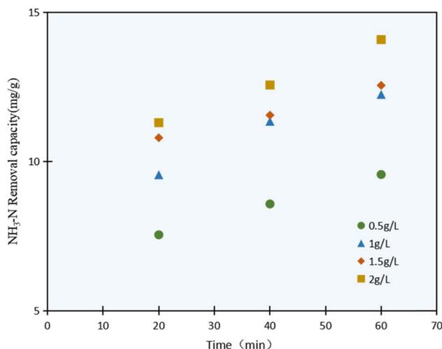
Fig. 4 NH<sub>3</sub>-N removal capacity with various C/TiO<sub>2</sub> dosages (AM1.5, 25 A, pH 10.0, C<sub>0</sub> = 50 mg L<sup>-1</sup>).
