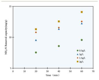
Fig. 4 NH<sub>3</sub>-N removal capacity with various C/TiO<sub>2</sub> dosages (AM1.5, 25 A, pH 10.0,  $C_0 = 50$  mg L<sup>-1</sup>).
