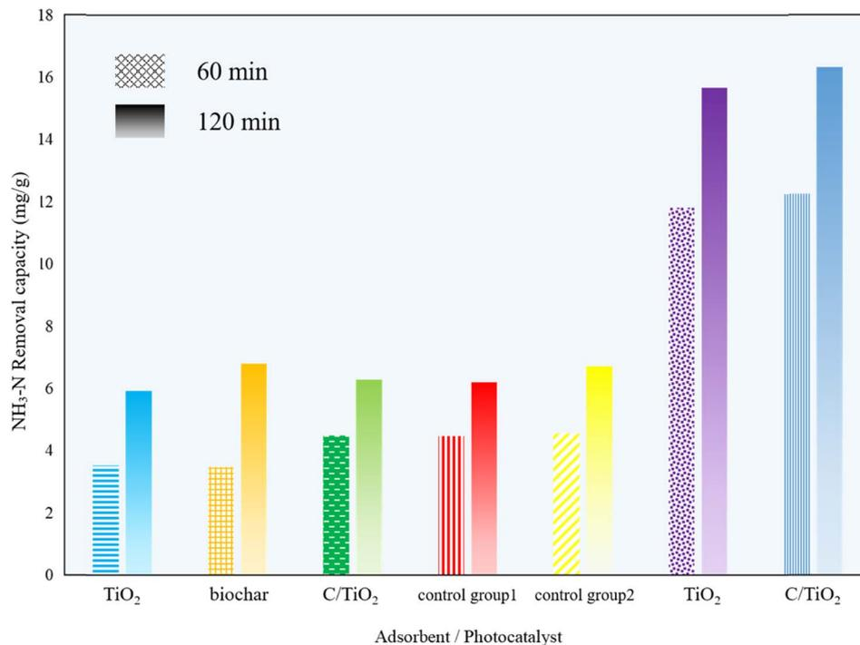
Fig. 1 NH<sub>3</sub>-N removal capacity under different reaction condition times (AM1.5, 25 A, 1 g L<sup>-1</sup> of photocatalyst, pH 10.0, C<sub>0</sub> = 50 mg L<sup>-1</sup>).
