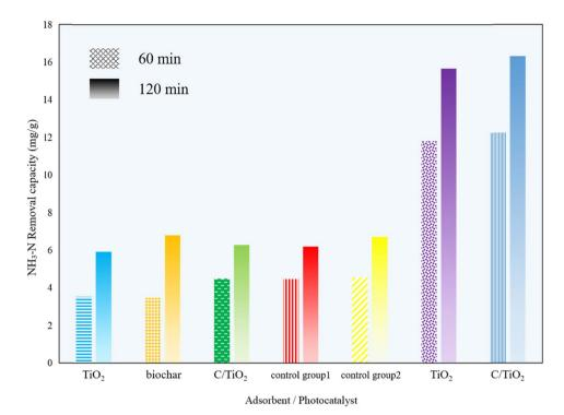
Fig. 1 NH<sub>3</sub>-N removal capacity under different reaction condition times (AM1.5, 25 A, 1 g  $L^{-1}$  of photocatalyst, pH 10.0,  $C_0 = 50$  mg  $L^{-1}$ ).
