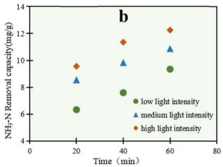
Fig. 2  $\,$  NH<sub>3</sub>–N removal capacity under different irradiation intensities by the C/TiO<sub>2</sub> photocatalysts, with varying the (a) light source (25 A, 1 g L<sup>-1</sup> C/TiO<sub>2</sub>, pH 10.0,  $C_0=50$  mg L<sup>-1</sup>); and (b) light intensity, from a low to high intensity of 50–100 mW cm<sup>-2</sup> (AM1.5, 1 g L<sup>-1</sup> C/TiO<sub>2</sub>, pH 10.0,  $C_0=50$  mg L<sup>-1</sup>).
