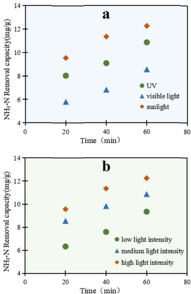
Fig. 2  $\text{NH}_3\text{-N}$  removal capacity under different irradiation intensities by the  $\text{C}/\text{TiO}_2$  photocatalysts, with varying the (a) light source (25 A,  $1 \text{ g L}^{-1} \text{ C}/\text{TiO}_2$ , pH 10.0,  $C_0 = 50 \text{ mg L}^{-1}$ ); and (b) light intensity, from a low to high intensity of  $50\text{--}100 \text{ mW cm}^{-2}$  (AM1.5,  $1 \text{ g L}^{-1} \text{ C}/\text{TiO}_2$ , pH 10.0,  $C_0 = 50 \text{ mg L}^{-1}$ ).
