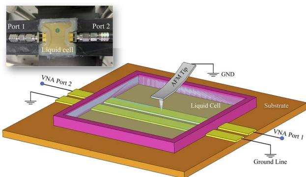
**Fig. 1** Schematic of an AFM-based iSMM: a planar waveguide – either a coplanar waveguide or a slot line – is used as a sample holder. Reflection and transmission coefficients are measured while a conductive grounded tip is scanned across the sample perturbing the field. The whole AFM tip is immersed in liquid (note: several details are not shown to simplify the schematic). (inset) Picture of the slot-line used in the reported experiments, highlighting the plastic container for liquid.
