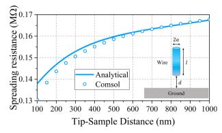
Fig. 4 Comparison of spreading resistance calculated from eqn (6) and from COMSOL for a cylinder in DMEM at 1.5 GHz.
