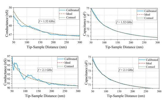
Fig. 7 Top left: comparison between expected ideal, Comsol and measured conductance in distilled water with a sphere 8 nm of radius, after calibration at 1.52 GHz as a function of the probe-metal distance; top right, same comparison for the capacitance; bottom left, comparison for the conductance at 2.1 GHz and bottom right comparison for the capacitance
