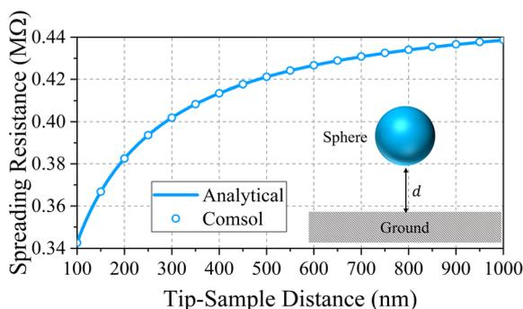
Fig. 3 Comparison of spreading resistance calculated from eqn (5) and from COMSOL for a sphere in DMEM at 1.5 GHz.
