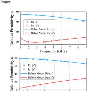
Fig. 2 Comparison between real and imaginary part of (top) DMEM and (bottom) distilled water permittivity as measured in ref. 7 and as fitted by eqn (8) and (9). Parameters in the text.
