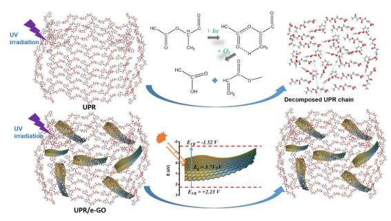
Fig. 9 Possible mechanism of enhancement UV resistance in UPR/e-GO nanocomposites compared to neat UPR.
