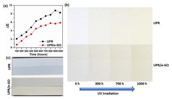
Fig. 10 Color change of materials after UV irradiation when measuring color (a) and artificial guartz stone samples (b and c).
