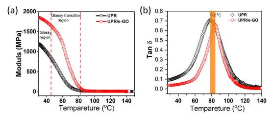
Fig. 8 Dynamic mechanical thermal analysis (DMA) spectra: (a) storage modulus (E') and (b) loss factor (tan  $\delta$ ) of UPR and UPR/e-GO.
