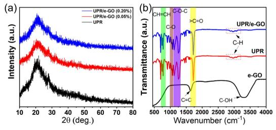
Fig. 3 XRD pattern of neat UPR and UPR/e-GO (a); FTIR spectra of e-GO, neat UPR and UPR/e-GO (b).
