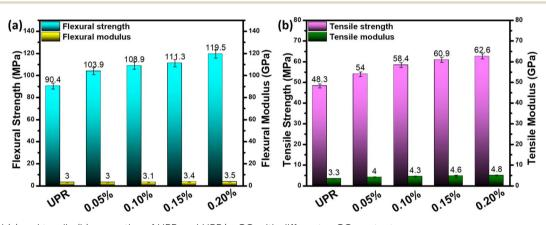
Fig. 5 Flexural (a) and tensile (b) properties of UPR and UPR/e-GO with different e-GO content.
