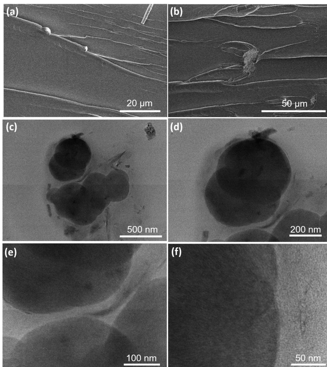
Fig. 2 SEM images of (a) neat UPR and (b) UPR/e-GO; HR-TEM images of (c–f) UPR/e-GO at different magnifications.
