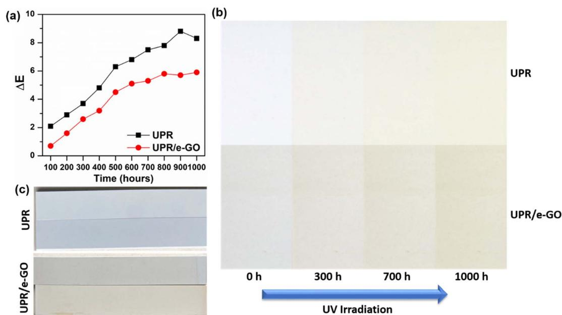
Fig. 10 Color change of materials after UV irradiation when measuring color (a) and artificial quartz stone samples (b and c).
