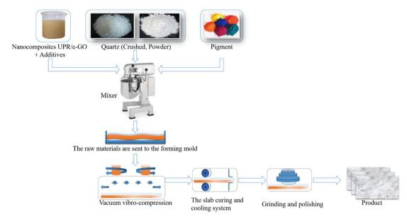
Scheme 2 Schematic illustration of the manufacturing process of grain-reinforced composites (quartz-based artificial stone).
