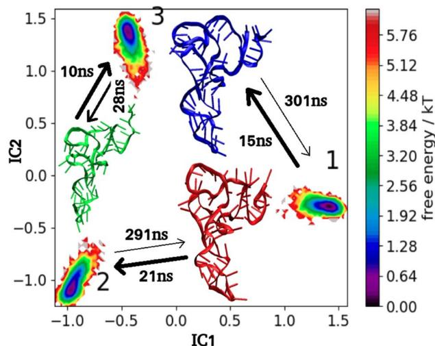
Fig. 13 MSM macrostates and MFPT rates for  $\text{tRNA}_3^{\text{Lys}}-1,5\text{T}$  system. The arrows show MFPT in ns. The metastable representative structures 1, 2 and 3 are shown in red, green and blue colors respectively.
