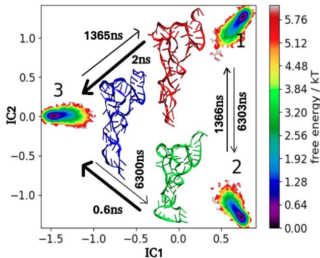
Fig. 12 MSM macrostates and MFPT rates for  $\text{tRNA}_3^{\text{Lys}}-1,4\text{T}$  system. The arrows show MFPT in ns. The metastable representative structures 1, 2 and 3 are shown in red, green and blue colors respectively.
