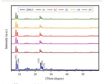
Fig. 2 XRD patterns of all the catalyst samples.
