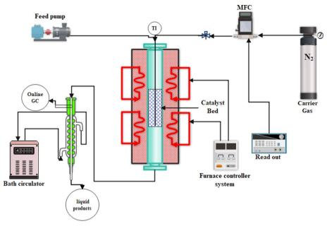
Fig. 1 Setup of catalytic cracking reactor to test the prepared catalytic samples.
