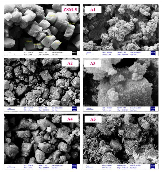
Fig. 6 FE-SEM images of the catalyst samples.
