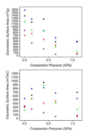
Fig. 3 Gravimetric (top) and volumetric (bottom) for UiO-66 (black) as compared to -NH<sub>2</sub> (blue), acetyl (green), 3,5,5-trimethylhexanoyl (red), and lauroyl-amide (purple) functionalized framework.
