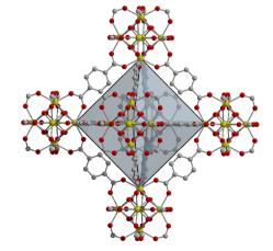
Fig. 1 A portion of the structure of UiO-66 where yellow, red, and gray spheres represent zirconium, oxygen, and carbon atoms, respectively. Hydrogen atoms have been omitted for clarity. UiO-66-NH $_2$  features disordered 2-position functionalization of terephthalic acid with  $-NH_2$ . These groups have also been omitted.
