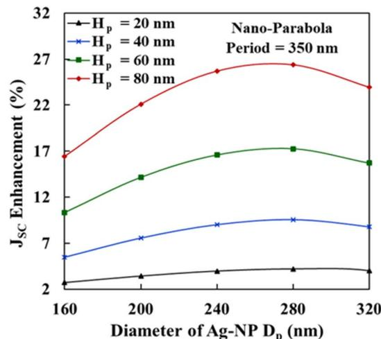
Fig. 7  $J_{SC}$  enhancement in the OSC by employing the 2D array of nano-parabolas on the top of back Ag layer as a function of back parabola diameter ( $D_p$ ) for varying height –  $H_p = 20$  nm, 40 nm, 60 nm, and 80 nm.
