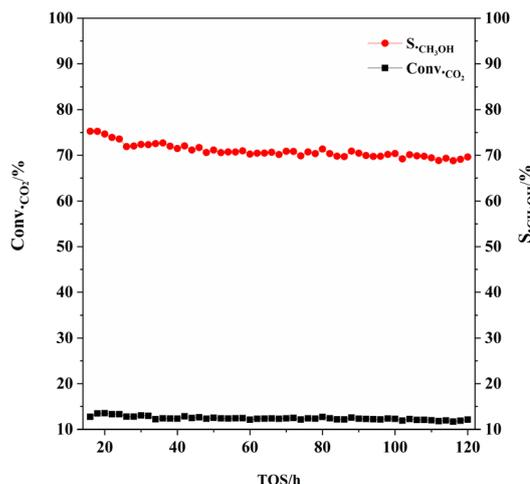
Fig. 9 The variation of catalytic performance of CZA-2%G catalyst during a TOS of 120 h. Reaction conditions: H<sub>2</sub> : CO<sub>2</sub> = 3 : 1, W/F = 10 g h mol<sup>-1</sup>, P = 3.0 MPa, T = 200 °C.
