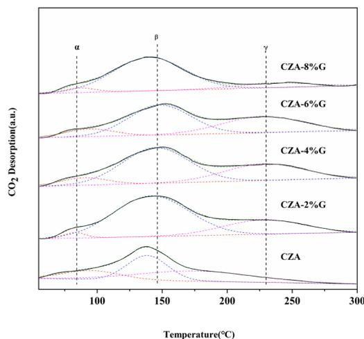
Fig. 7 CO<sub>2</sub>-TPD profiles of the CZA and CZA-G catalyst samples.
