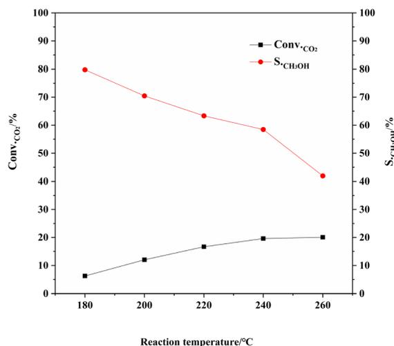
Fig. 8 Catalytic performance of CZA-2%G catalyst at different reaction temperatures. Reaction conditions: H<sub>2</sub> : CO<sub>2</sub> = 3 : 1, W/F = 10 g h mol<sup>-1</sup>, P = 3.0 MPa, T = 180 °C/200 °C/220 °C/240 °C/260 °C.
