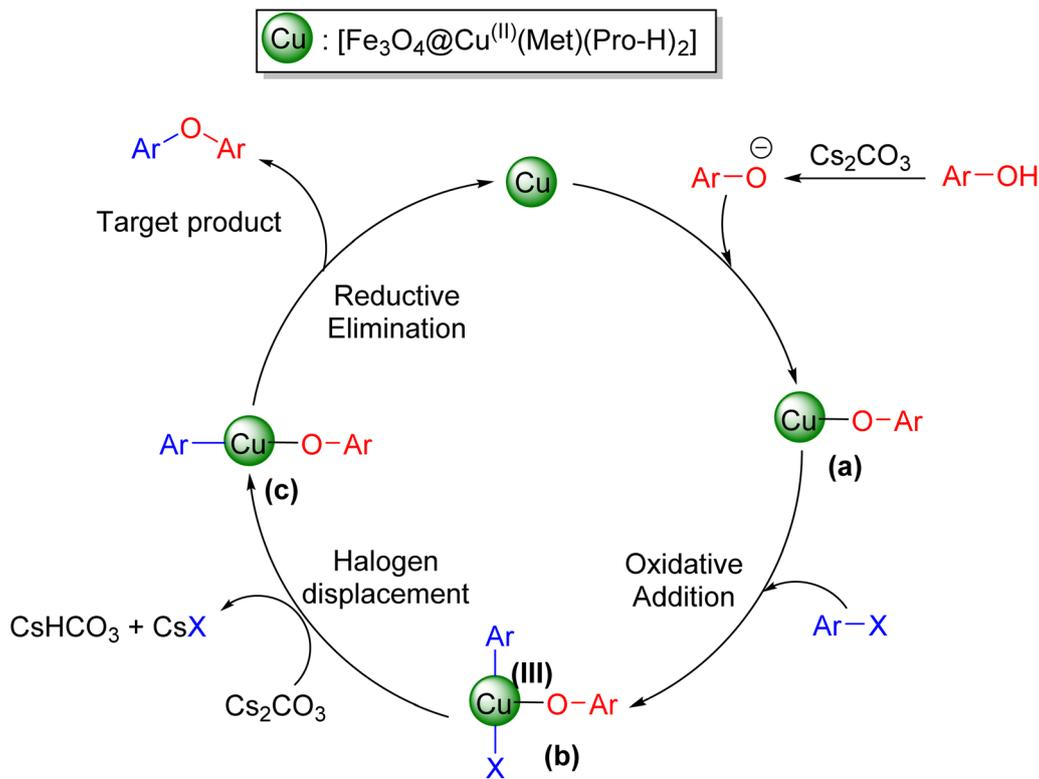
Scheme 2 The proposed mechanism for the Ullmann synthesis of diaryl ethers over [Fe<sub>3</sub>O<sub>4</sub>@Cu<sup>(II)</sup>(Met)(Pro-H)<sub>2</sub>] catalyst.
