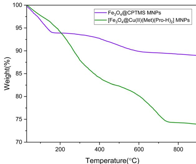
Fig. 3 TGA analysis of Fe<sub>3</sub>O<sub>4</sub>@CPTMS and [Fe<sub>3</sub>O<sub>4</sub>@Cu(II)(Met)(Pro-H)<sub>2</sub>] MNPs.
