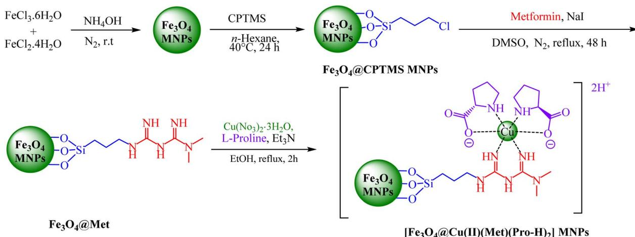
Scheme 1 Synthesis of [Fe<sub>3</sub>O<sub>4</sub>@Cu(II)(Met)(Pro-H)<sub>2</sub>] MNPs.
