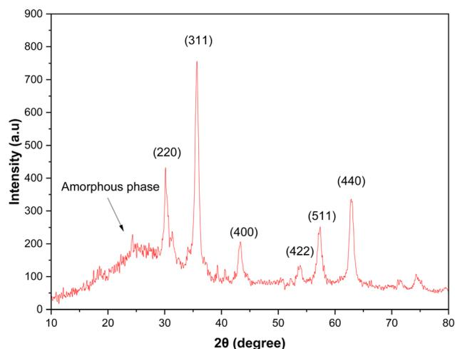
Fig. 2 XRD pattern of [Fe<sub>3</sub>O<sub>4</sub>@Cu(II)(Met)(Pro-H)<sub>2</sub>] MNPs.
