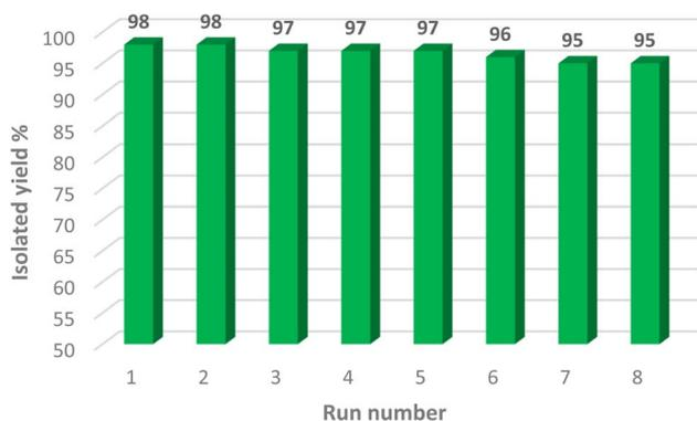
Fig. 9 Reusability of [Fe<sub>3</sub>O<sub>4</sub>@Cu<sup>(II)</sup>(Met)(Pro-H)<sub>2</sub>] MNPs.
