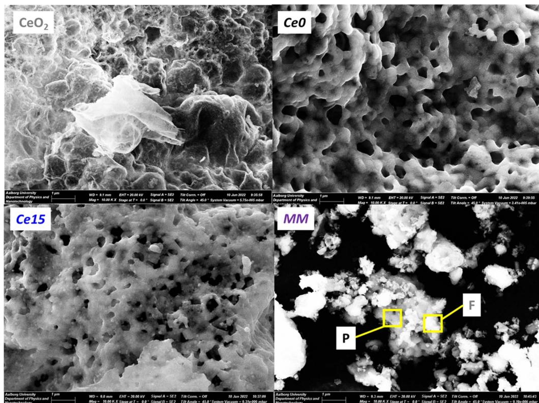
Fig. 4 SEM images of  $\text{CeO}_2$ ,  $\text{Ce0}$ ,  $\text{Ce15}$  and  $\text{MM}$ . In  $\text{MM}$ , the darker perovskite (P) and lighter fluorite (F) grains are highlighted in agreement with the EDX results in Fig. S6.†
