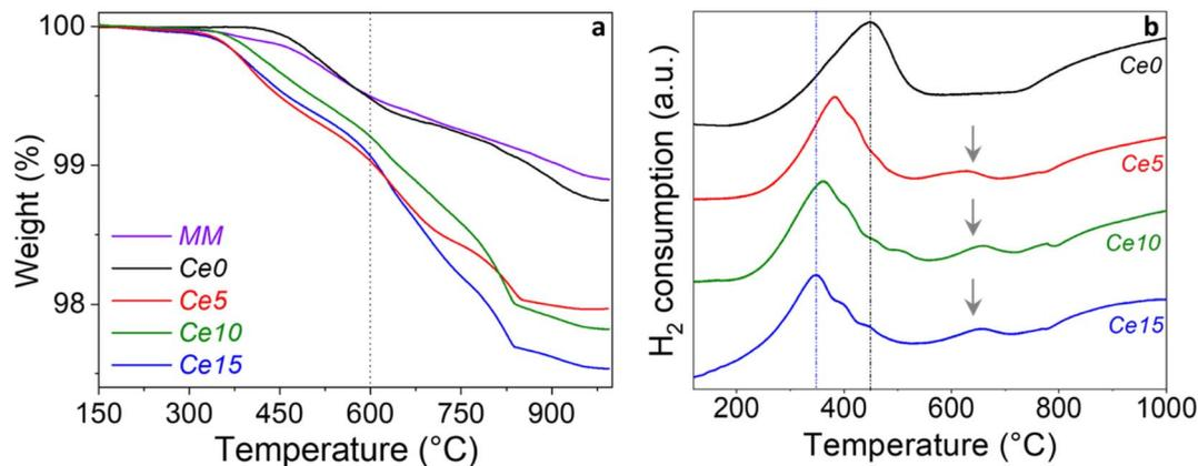
Fig. 5 (a) TGA graph of the investigated  $\text{SrFeO}_3$ -based powders prepared with different cerium excess and comparison with the mechanical mixture; (b) comparison between TPR of  $\text{Ce0}$ ,  $\text{Ce5}$ ,  $\text{Ce10}$  and  $\text{Ce15}$ . The TPR peak at around 650 °C is evidenced by an arrow only in the powders with some cerium excess.
