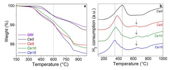
Fig. 5 (a) TGA graph of the investigated  $SrFeO_3$ -based powders prepared with different cerium excess and comparison with the mechanical mixture; (b) comparison between TPR of *CeO*, *Ce5*, *Ce10* and *Ce15*. The TPR peak at around 650 °C is evidenced by an arrow only in the powders with some cerium excess.
