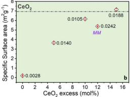
Fig. 3 (a) Microstrain trend of Ce-doped SrFeO<sub>3</sub> perovskite (P) and CeO<sub>2</sub> fluorite (F) structures with increasing cerium excess; (b) trend of surface area with increasing cerium excess; the numbers close to each symbol indicate relative cumulative pore volume on desorption (cm<sup>3</sup> g<sup>-1</sup>).
