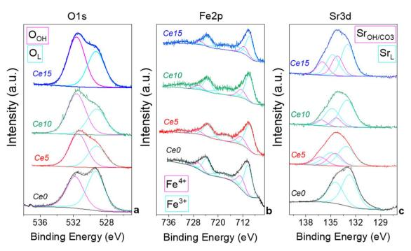
Fig. 2 X-ray photoelectron spectroscopy spectra of the investigated samples: (a) O 1s region, where  $O_L$  and  $O_{OH}$  represent the lattice oxygen and the surface oxygen, respectively; (b) Fe 2p region where Fe<sup>4+</sup> and Fe<sup>3+</sup> contributions are evidenced; (c) Sr 3d region., whereas Sr<sub>L</sub> and Sr<sub>OH/CO3</sub> represent the Sr in the perovskite structure and the Sr in the SrCO<sub>3</sub> structure, respectively.
