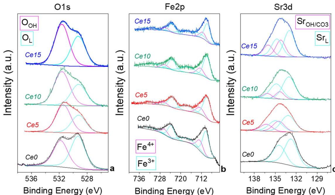
Fig. 2 X-ray photoelectron spectroscopy spectra of the investigated samples: (a) O 1s region, where  $O_L$  and  $O_{OH}$  represent the lattice oxygen and the surface oxygen, respectively; (b) Fe 2p region where  $Fe^{4+}$  and  $Fe^{3+}$  contributions are evidenced; (c) Sr 3d region, whereas  $Sr_L$  and  $Sr_{OH/CO_3}$  represent the Sr in the perovskite structure and the Sr in the  $SrCO_3$  structure, respectively.
