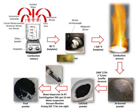
Scheme 1 Schematical description of the solution combustion synthesis procedure used for the preparation of Ce-doped SrFeO<sub>3</sub> with cerium excess.
