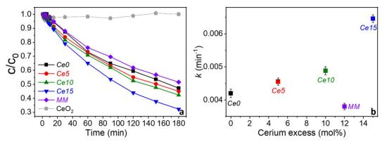
Fig. 6 (a) Thermocatalytic abatement of bisphenol A (initial concentration 10 mg  $L^{-1}$ ) at 50 °C for perovskites (1 g  $L^{-1}$ ) with excess ceria and the mechanical mixture (*MM*) and (b) change in kinetic constant (*k*) with increasing excess ceria and comparison with the mechanical mixture. Errors in (a) are smaller than the size of the symbols, whereas in (b) the errors are indicated in the graph for each *k* value.
