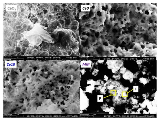
Fig. 4 SEM images of  $CeO_2$ , CeO, CeO, CeO, CeO, and MM. In MM, the darker perovskite (P) and lighter fluorite (F) grains are highlighted in agreement with the EDX results in Fig. S6.†
