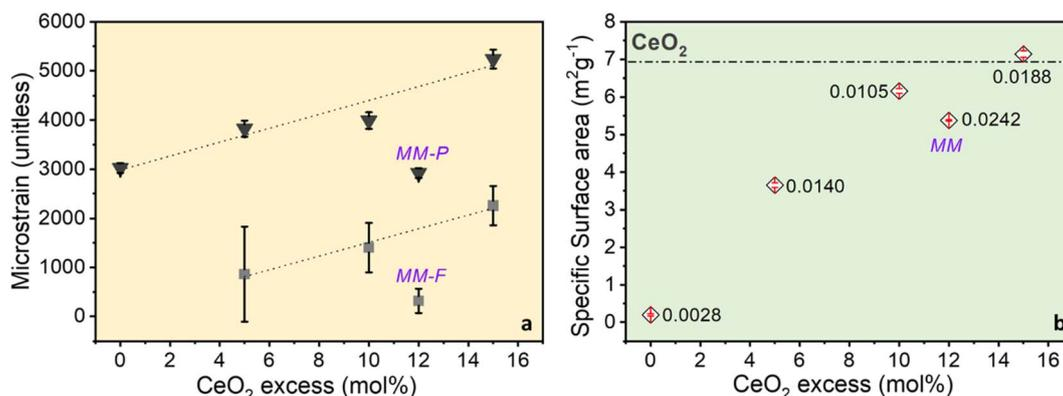
Fig. 3 (a) Microstrain trend of Ce-doped  $\text{SrFeO}_3$  perovskite (P) and  $\text{CeO}_2$  fluorite (F) structures with increasing cerium excess; (b) trend of surface area with increasing cerium excess; the numbers close to each symbol indicate relative cumulative pore volume on desorption ( $\text{cm}^3 \text{g}^{-1}$ ).
