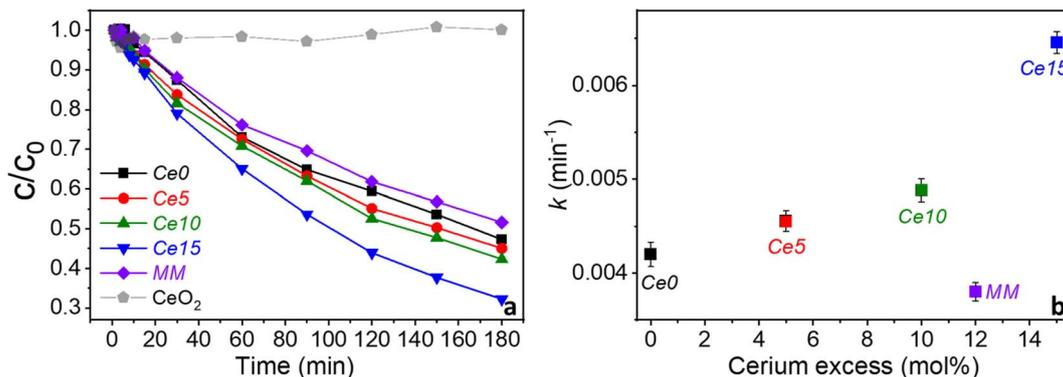
Fig. 6 (a) Thermocatalytic abatement of bisphenol A (initial concentration  $10 \text{ mg L}^{-1}$ ) at  $50^\circ \text{C}$  for perovskites ( $1 \text{ g L}^{-1}$ ) with excess ceria and the mechanical mixture (MM) and (b) change in kinetic constant ( $k$ ) with increasing excess ceria and comparison with the mechanical mixture. Errors in (a) are smaller than the size of the symbols, whereas in (b) the errors are indicated in the graph for each  $k$  value.
