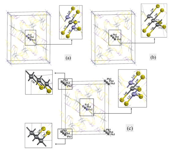
Fig. 6 Models of the single Pb substitution systems of jamesonite: (a) one Pb atom substitution; (b) two Pb atoms substitution; (c) three Pb atoms substitution
