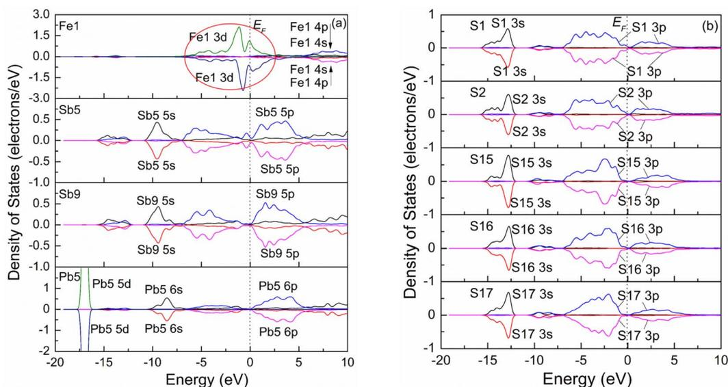
Fig. 3 Spin polarizing partial density of states of pure jamesonite: (a) metal atoms; (b) S atoms.
