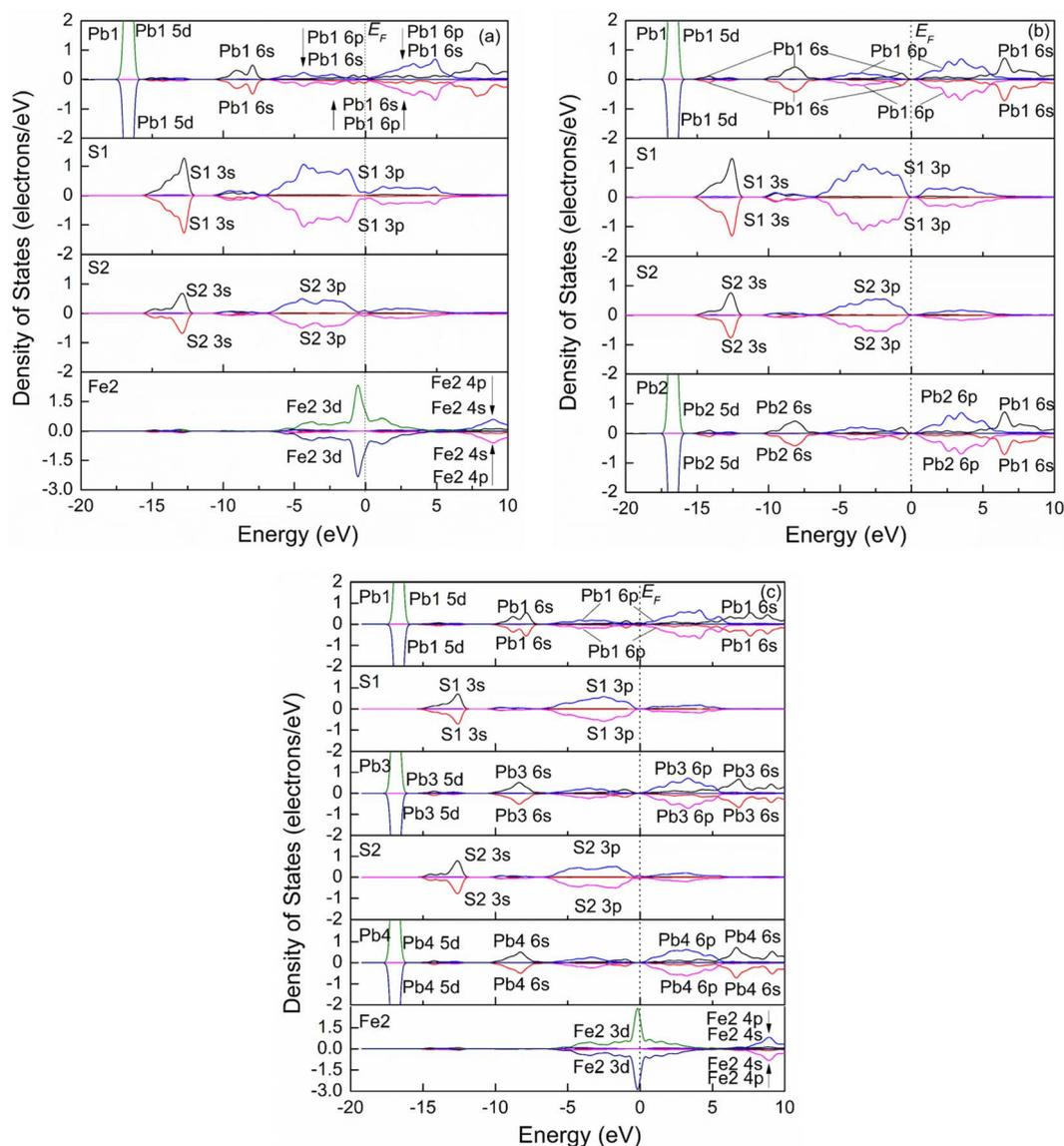
Fig. 7 Spin partial density of states of jamesonite of the Pb substitution systems. (a) One Pb atom substitution; (b) two Pb atoms substitution; (c) three Pb atoms substitution.
