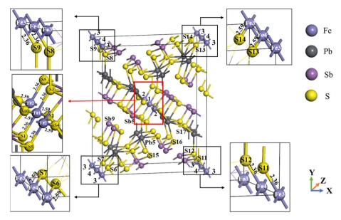
Fig. 1 Model of the jamesonite structure.
