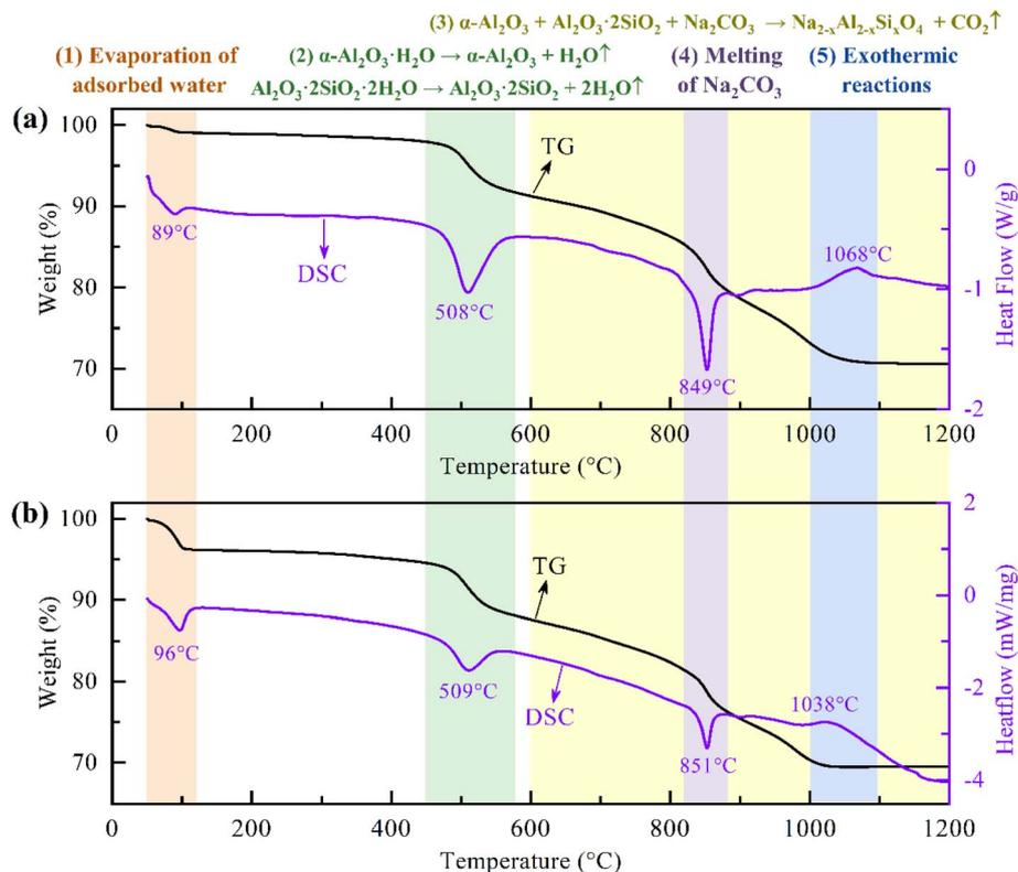
Fig. 4 TG and DSC curves of the mixture of bauxite and  $\text{Na}_2\text{CO}_3$  with  $N/(A + S) = 1$  under nitrogen (a) and air (b)<sup>37</sup> atmospheres.
