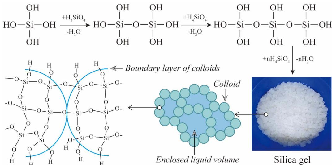
Fig. 11 Diagram of the formation mechanism of silica gel.<sup>43</sup>
