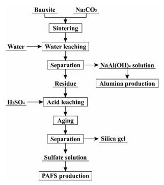
Fig. 1 Flowsheet for extraction of alumina and silica from high-silica bauxite.
