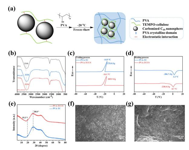
Fig. 2 (a) Schematic illustration of the fabrication process of PVA-TCCS hydrogels. (b) FTIR spectra of PVA hydrogel, PVA-TC hydrogel, and PVA-TCCS hydrogel DSC curves of PVA-TC hydrogel and PVA-TCCS hydrogel during (c) the cooling process and (d) the heating process. (e) XRD patterns of PVA-TC hydrogel and PVA-TCCS hydrogel. SEM images of the freeze-dried (f) PVA-TC hydrogel and (g) PVA-TCCS hydrogel.
