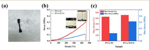
Fig. 3 (a) Photo of the PVA-TC hydrogel (right) and PVA-TCCS hydrogel (left) samples for stretching tests. (b) Strain-stress curves of PVA-TC and PVA-TCCS hydrogels. (c) The max strain and max stress values obtained from the strain-stress curves.
