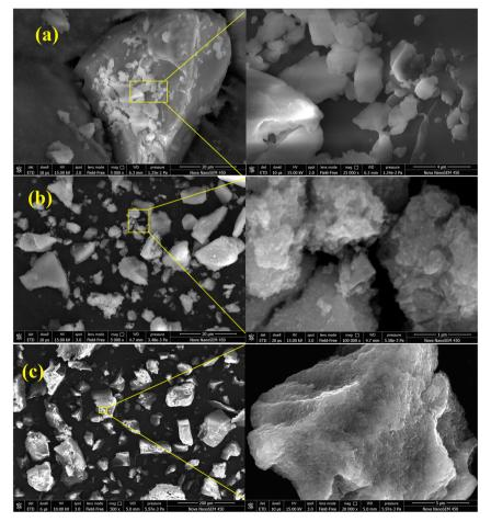
Fig. 2 SEM images of (a)  $\beta$ -CD-E-T, (b) ZnFe<sub>2</sub>O<sub>4</sub>, and (c)  $\beta$ -CD-E-T/ZnFe<sub>2</sub>O<sub>4</sub>.
