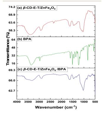
Fig. 1 FTIR spectrum of (a)  $\beta$ -CD-E-T/ZnFe<sub>2</sub>O<sub>4</sub>, (b) BPA, and (c)  $\beta$ -CD-E-T/ZnFe<sub>2</sub>O<sub>4</sub> after BPA adsorption.
