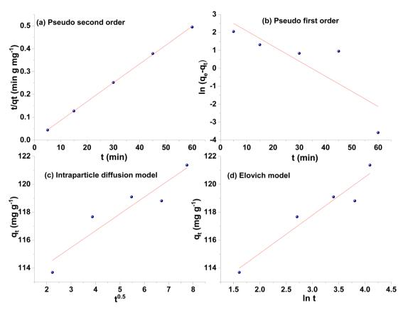
Fig. 6 Adsorption kinetics plots of BPA adsorption onto  $\beta$ -CD-E-T/ZnFe<sub>2</sub>O<sub>4</sub>: (a) pseudo-second-order, (b) pseudo-first-order, (c) intraparticle diffusion, and (d) Elovich plot.
