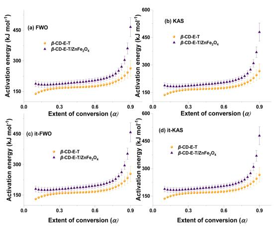
Fig. 4 Variation in the activation energy of the thermal decomposition of  $\beta$ -CD-E-T and  $\beta$ -CD-E-T/ZnFe<sub>2</sub>O<sub>4</sub> calculated using (a) FWO, (b) KAS, (c) it-FWO, and (d) it-KAS with the extent of conversion.
