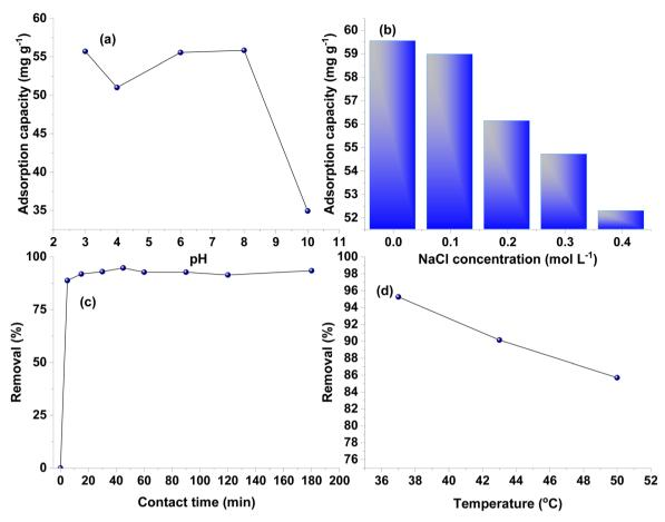
Fig. 5 Effect of (a) pH, (b) ionic salt concentration, (c) contact time, and (d) temperature on the adsorption of BPA by  $\beta$ -CD-E-T/ZnFe<sub>2</sub>O<sub>4</sub> from aqueous solution.
