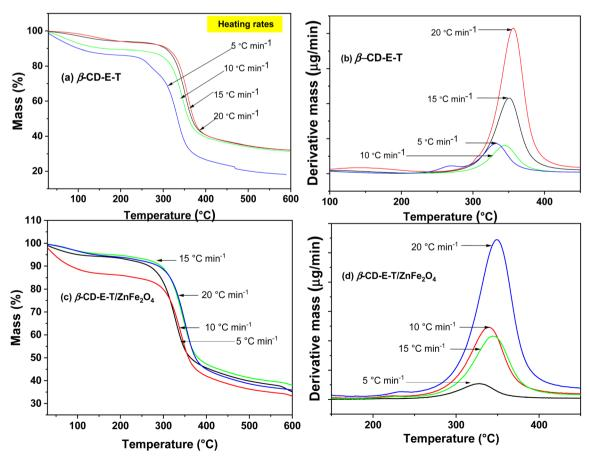
Fig. 3 (a) TG curve of β-CD-E-T, (b) DTG curve of β-CD-E-T, (c) TG curve of β-CD-E-T/ZnFe<sub>2</sub>O<sub>4</sub>, and (d) DTG curve of β-CD-E-T/ZnFe<sub>2</sub>O<sub>4</sub>.
