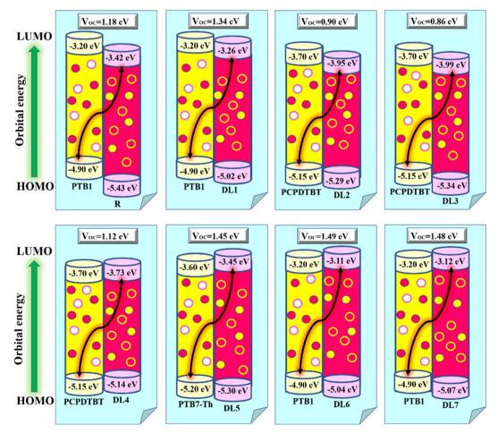
Fig. 8  $V_{\rm OC}$  of designed acceptors (DL1-DL7) against donor J61.
