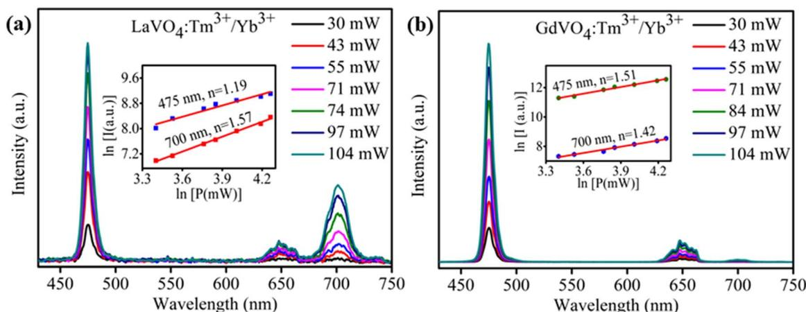
Fig. 4 Pump power dependent UC spectra of Tm<sup>3+</sup>/Yb<sup>3+</sup> codoped (a) LaVO<sub>4</sub> (b) GdVO<sub>4</sub> phosphors. Inset of both figures represent the  $\ln$ - $\ln$  plot of UC emission intensity versus excitation power.
