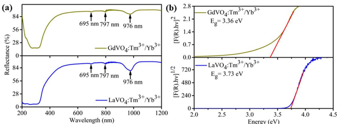
Fig. 2 (a) UV-vis-NIR absorption spectra in diffuse reflectance mode of  $\text{Tm}^{3+}/\text{Yb}^{3+}$  codoped monazite type  $\text{LaVO}_4$  and zircon type  $\text{GdVO}_4$  phosphors; (b) Kubelka–Munk plots to estimate the optical band gap energies of the synthesized phosphors.
