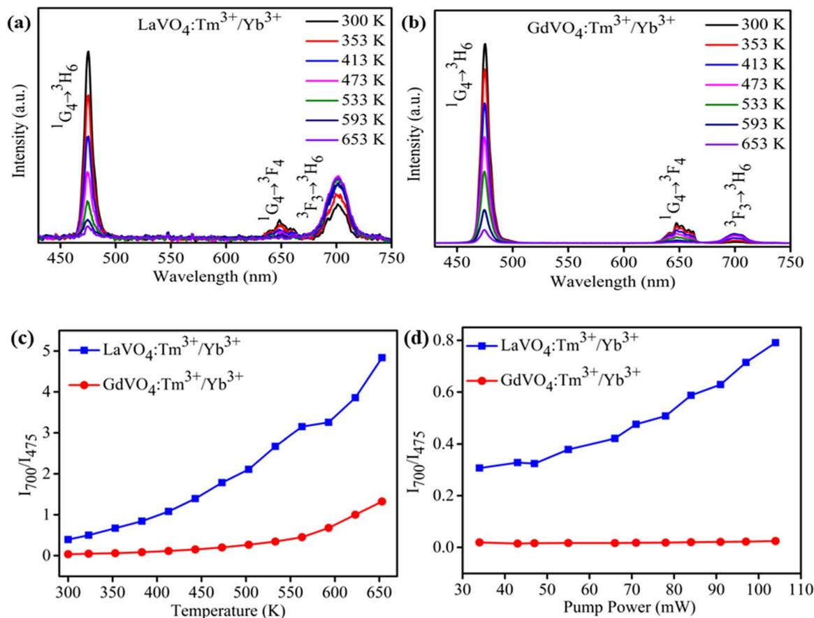
Fig. 5 (a) Temperature dependent UC spectra upon 980 nm laser excitation in temperature range 300–653 K of (a)  $\text{Tm}^{3+}/\text{Yb}^{3+}:\text{LaVO}_4$  (b)  $\text{Tm}^{3+}/\text{Yb}^{3+}:\text{GdVO}_4$  phosphors. Variation in the ratio of red/blue emission band ( $I_{700}/I_{475}$ ) in both the phosphors at varying (c) temperature (d) pump power.
