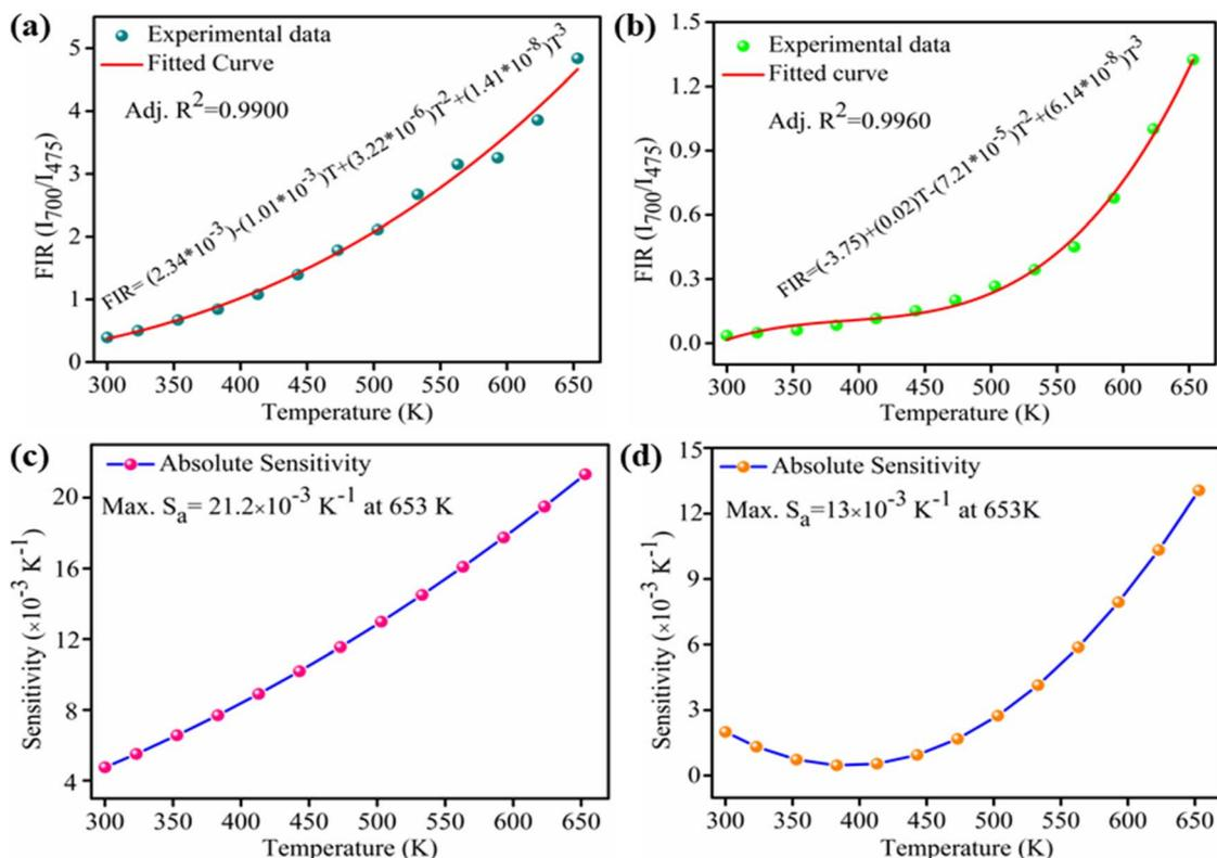
Fig. 7 Polynomial fitting of FIR data of NTCLs ( $^3F_3$  and  $^1G_4$ ) as a function of temperature for (a)  $Tm^{3+}/Yb^{3+}$ :  $LaVO_4$  (b)  $Tm^{3+}/Yb^{3+}$ :  $GdVO_4$  phosphors; absolute sensitivity as a function of temperature for (c)  $Tm^{3+}/Yb^{3+}$ :  $LaVO_4$  (d)  $Tm^{3+}/Yb^{3+}$ :  $GdVO_4$  phosphors.
