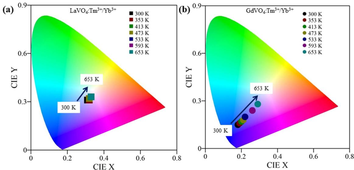
Fig. 8 CIE colour chromaticity diagram of (a)  $LaVO_4$ : 0.3 mol%  $Tm^{3+}/5$  mol%  $Yb^{3+}$  (b)  $GdVO_4$ : 0.3 mol%  $Tm^{3+}/5$  mol%  $Yb^{3+}$  phosphors. Colour change is more prominent in  $GdVO_4$  phosphor.
