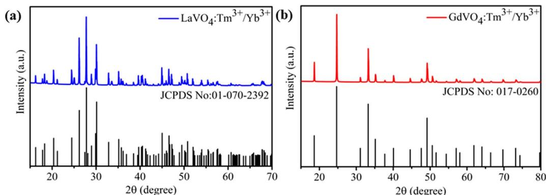
Fig. 1 X-ray diffraction pattern of 0.3 mol%  $\text{Tm}^{3+}$ /5 mol%  $\text{Yb}^{3+}$  codoped (a) monazite type  $\text{LaVO}_4$  (b) zircon type  $\text{GdVO}_4$  phosphors.
