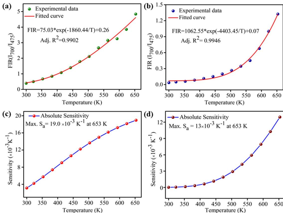
Fig. 6 Exponential fitting of FIR data of non-thermally coupled levels ( $^3F_3$  and  $^1G_4$ ) as a function of temperature for (a)  $Tm^{3+}/Yb^{3+}$ :  $LaVO_4$  (b)  $Tm^{3+}/Yb^{3+}$ :  $GdVO_4$  phosphors; absolute sensitivity as a function of temperature for (c)  $Tm^{3+}/Yb^{3+}$ :  $LaVO_4$  (d)  $Tm^{3+}/Yb^{3+}$ :  $GdVO_4$  phosphors.
