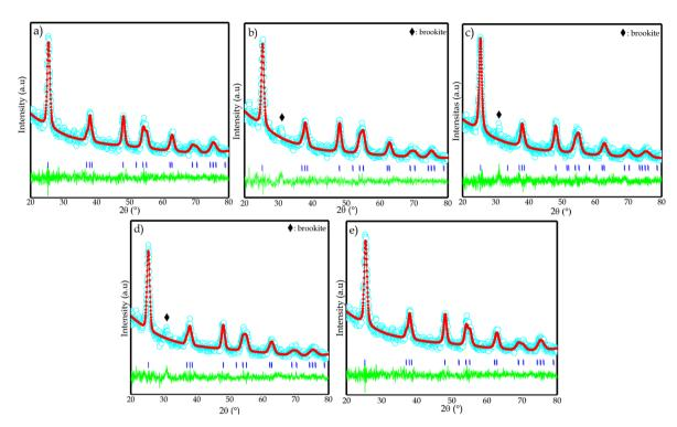
Fig. 6 Le Bail plot of samples: (a) CTO, (b) NCT0.25, (c) NCT0.5, (d) NCT0.75, and (e) NCT1 based on XRD data with space group I4<sub>1</sub>/amdS.
