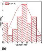
Fig. 3 FESEM images and particle size distribution of samples: (a) NTi0.75 and (b) NCT0.75.
