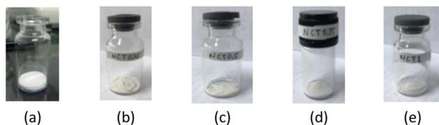
Fig. 2 Synthesized porous TiO<sub>2</sub> and N-doped porous TiO<sub>2</sub> nanoparticle samples: (a) CTO, (b) NCT0.25, (c) NCT0.5, (d) NCT0.75, and (e) NCT1.
