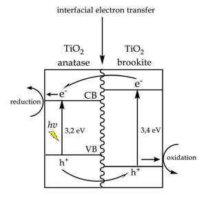
Fig. 14 Charge transfer scheme at anatase/brookite  ${\rm TiO_2}$  heterojunction.
