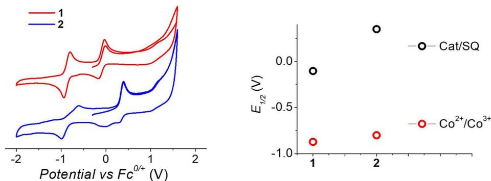
Fig. 3 Voltammograms of acetonitrile solutions of the complexes, measured with a 100 mV s<sup>-1</sup> sweeping rate, (left) and corresponding potentials (right panel).
