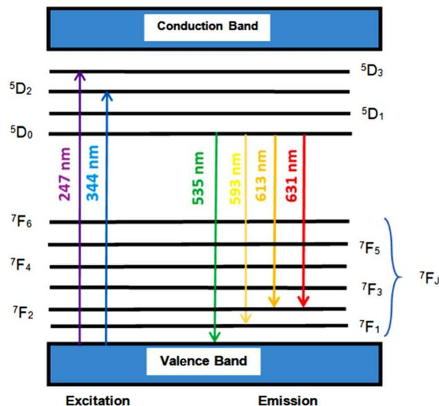
Fig. 7 Energy level diagram of  $\text{CaY}_2\text{O}_4:\text{Eu}^{3+}$ .
