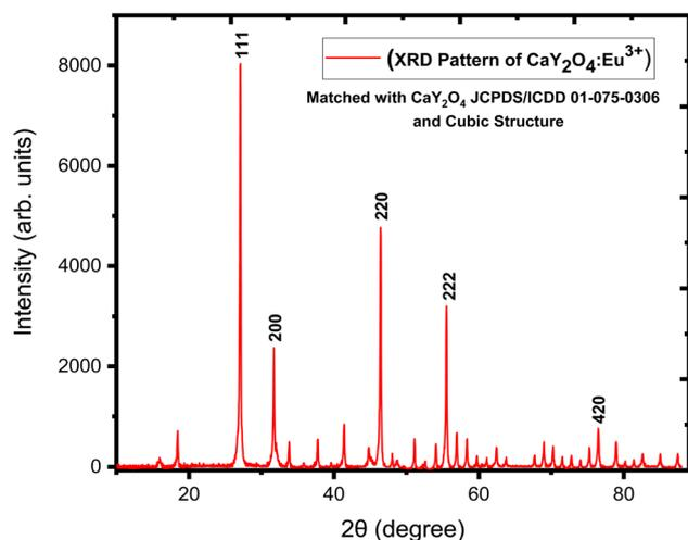
Fig. 2 XRD pattern of CaY<sub>2</sub>O<sub>4</sub>:Eu<sup>3+</sup>.Table 1 Calculation of crystallite size of CaY<sub>2</sub>O<sub>4</sub>:Eu<sup>3+</sup> phosphor
