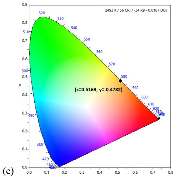
Fig. 6 (a) PL excitation spectra of  $\text{CaY}_2\text{O}_4:\text{Eu}^{3+}$  at 2.0 mol%. (b) PL emission curve of  $\text{CaY}_2\text{O}_4:\text{Eu}^{3+}$  for (0.1–2.5) mol%. (c) Commission Internationale de l'Eclairage (CIE 1931) of  $\text{CaY}_2\text{O}_4:\text{Eu}^{3+}$  for 2.5 mol% ( $x = 0.5169$ ,  $y = 0.4782$ ).
