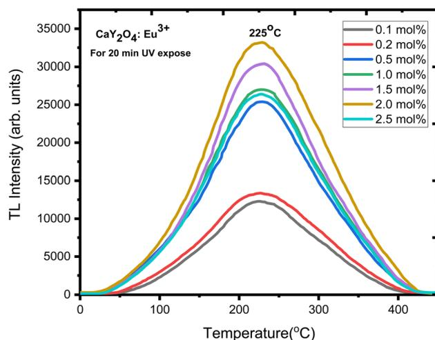
Fig. 8 TL glow curve analysis of  $\text{CaY}_2\text{O}_4:\text{Eu}^{3+}$ .
