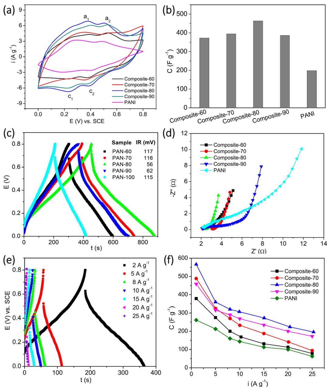
Fig. 6 Electrochemical properties of the ternary composites: (a) CV plots at a scan rate of 10 mV s<sup>-1</sup>, (b) specific capacitance at the scan rate of 10 mV s<sup>-1</sup>, (c) GCD plots at an applied current of 1 A g<sup>-1</sup>, (d) Nyquist type impedance spectra, (e) GCD plots of the typical composite-80 at various applied currents, and (f) the dependence of the specific capacitance on the applied current.
