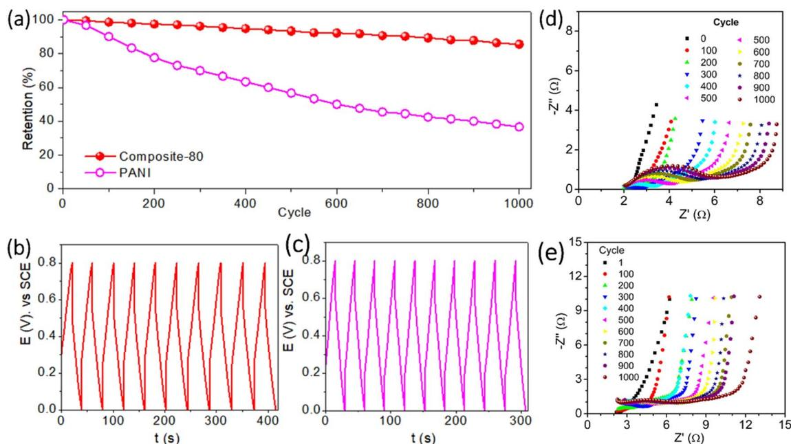
Fig. 8 (a) Long term-cyclability performance of composite-80 and PANI for 1000 cycles at an applied current of  $15 \text{ A g}^{-1}$  and the relevant GCD plots of (b) composite-80 and (c) PANI for the initial 10 cycles. Change in the Nyquist plots of (d) composite-80 and (e) PANI during cycling test.
