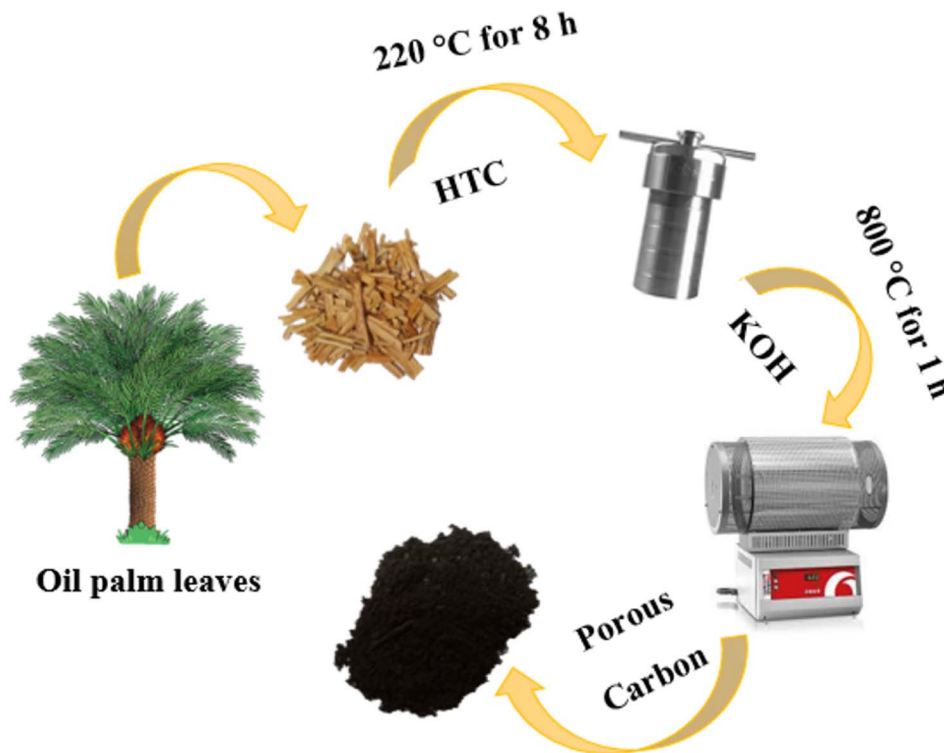
Fig. 1 Schematic illustration of the synthesis of oil palm leaf-derived hierarchical porous carbon.
