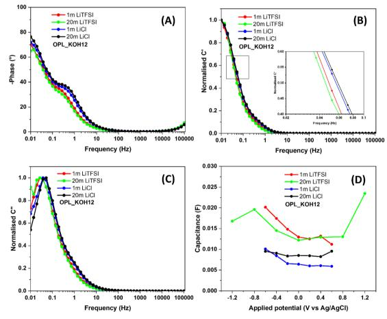
Fig. 5 (A) Bode plots of OPL\_KOH12 (all results are tested in 1 m, 20 m LiTFSI and 1 m, 20 m LiCl), (B) real and (C) imaginary parts of the normalized capacitances as a function of frequencies (all above results were tested in different electrolytes), (D) the capacitance of OPL\_KOH12 vs. applied voltage in different electrolytes (the capacitance of the electrode was calculated from the EIS measurement using eqn (S3)†).
