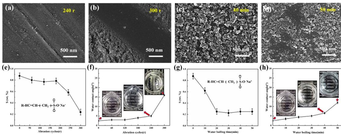
Fig. 4 Surface SEM images of the PAA-SiO<sub>2</sub> coatings after the Taber abrasion test for (a) 240 r cycles and (b) 300 r cycles. Surface SEM images of the PAA-SiO<sub>2</sub> coatings after boiling immersion test for (c) 40 min and (d) 50 min. Change in (e) sulfur content and (f) wettability of surfactant during Taber abrasion test. Change in (g) sulfur content and (h) wettability of surfactant during boiling immersion test.
