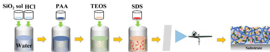
Fig. 1 Schematic of detailed manufacturing process.
