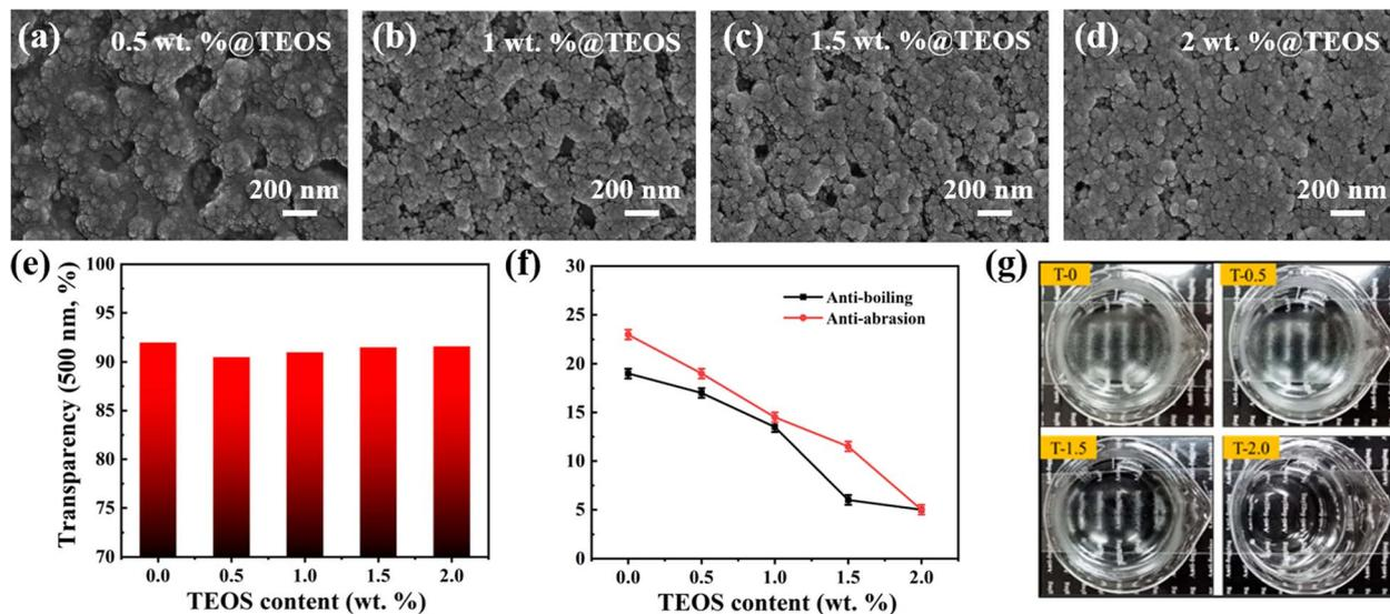
Fig. 5 Surface SEM images of the PAA-TEOS-SiO<sub>2</sub> coating with different mass ratios of TEOS: (a) 0.5 wt%, (b) 1 wt%, (c) 1.5 wt%, and (d) 2 wt%. (e) Transparency of the PAA-TEOS-SiO<sub>2</sub> coating with different TEOS contents. (f) Wettability changes after anti-boiling and anti-abrasion tests and (g) anti-fogging performance of the PAA-TEOS-SiO<sub>2</sub> coating with different TEOS contents.
