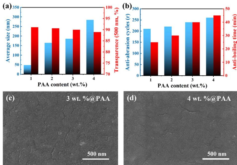
Fig. 3 (a) Average size and transparency of the PAA-SiO<sub>2</sub> SHPL coating at different mass ratios of PAA. (b) Anti-abrasion cycles and anti-boiling time of PAA-SiO<sub>2</sub> coatings at different mass ratios of PAA. SEM surface image of PAA-SiO<sub>2</sub> coating at (c) 3 wt% and (d) 4 wt% PAA mass ratio.
