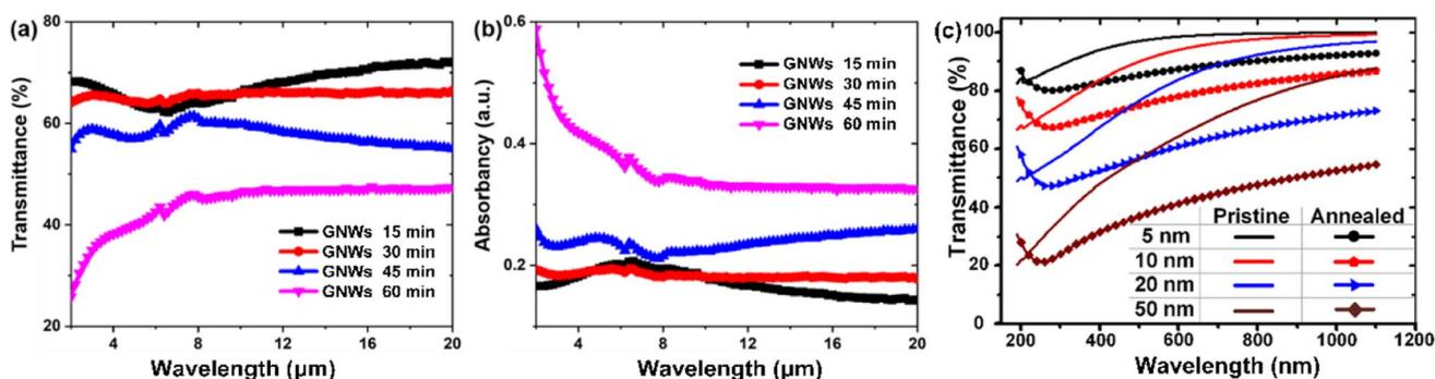
Fig. 6 Absorption spectra of GNWs with different growth time. (a) Transmittance; (b) absorbance; (c) optoelectronic properties of the DLC interlayer with different thicknesses before and after annealing. Copyright © 2021, American Chemical Society.
