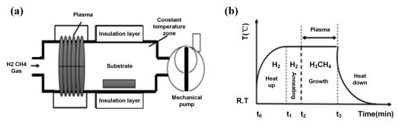
Fig. 3 Growth process of GMWs. (a) Schematic diagram of RF-PECVD equipment for the growth of GNWs. (b) Schematic illustrating the preparation process of GNWs.
