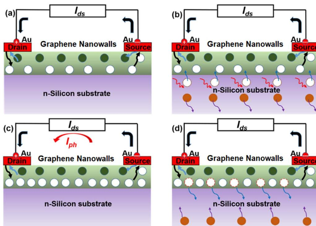
Fig. 14 Photogating effect of GNWs/semiconductor heterojunction. (a) Dark current under an external bias due to intrinsic carriers in GNWs; (b) incident photons generate electron–hole pairs in the silicon; (c) these injected carriers gate the GNWs channel; (d) at the end of their lifetime, these carriers recombine back into silicon.
