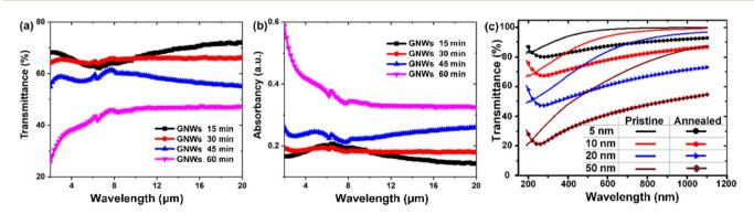
Fig. 6 Absorption spectra of GNWs with different growth time. (a) Transmittance; (b) absorbancy; (c) optoelectronic properties of the DLC interlayer with different thicknesses before and after annealing. Copyright © 2021, American Chemical Society.
