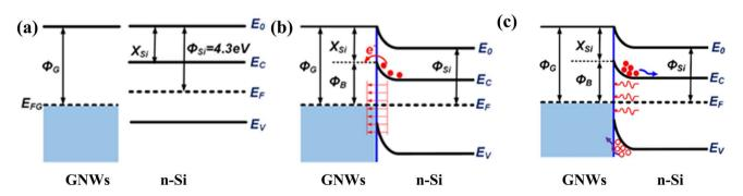
Fig. 9 Energy band structure of GNWs/Si. (a) Uncontacted; (b) contacted; (c) schematic diagram of energy band structure of GNWs/Si heterojunction. Copyright © 2019, American Chemical Society
