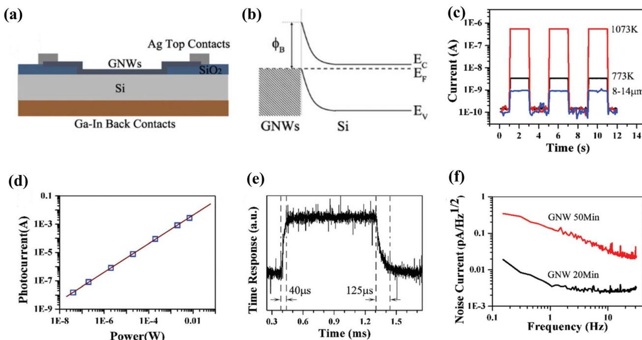
Fig. 10 GNWs-based photovoltaic detectors. (a) Schematic representation of the GNWs/Si heterojunction detector structure; (b) illustration of the energy band diagram of the device; (c) device response under 8–14  $\mu\text{m}$  laser excitation; (d) photocurrent response of the device at varying optical power levels; (e) response time characteristics of the device; (f) noise current associated with the device. Copyright © 2017, Royal Society of Chemistry.
