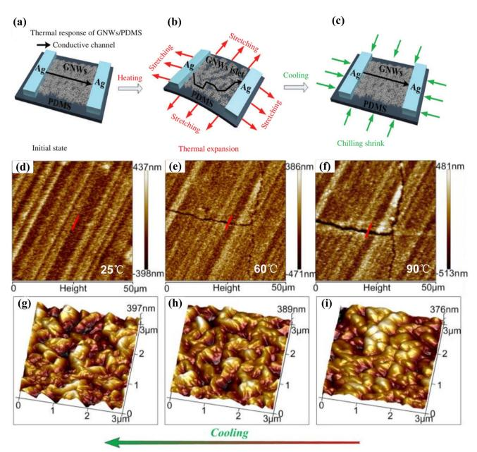
Fig. 18 GNWs-based photothermal detector. (a) – (c) Schematic diagram of the thermal response of GNWs/PDMS composites. Copyright © 2018, De Gruyter (d) – (f) surface morphology change of GNWs film under different temperature from 25 to 90 °C. AFM image of cracks evolution on GNWs film (50  $\times$  50  $\mu$ m) (q) – (i) the AFM cross-section of crack region (3  $\mu$ m). Copyright © 2011, RSC Publishing.
