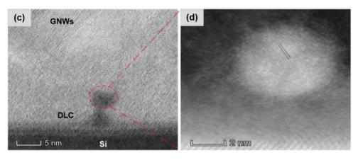
Fig. 8 Interface adhesion between GNWs and silicon substrate. (a) Cross-sectional SEM image of Si/GNWs; (b) micropattern of Si/GNWs. (c) and (d) high-magnification cross-sectional TEM images of Si/DLC/GNWs. Copyright © 2021, American Chemical Society.
