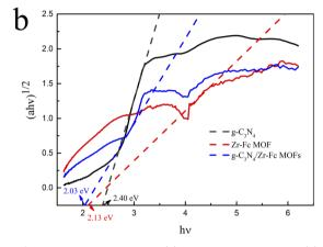
Fig. 3 Solid UV diffuse reflection (a) and band gap diagram (c) of g- $C_3N_4$ , Zr-Fc MOF, and g- $C_3N_4/Zr$ -Fc MOF.
