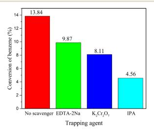
Fig. 6 Free-radical-trapping experiments. Reaction conditions: catalyst (1.5 mg mL $^{-1}$ ), benzene (1.6 mL, 18.05 mmol), H $_2$ O $_2$  (30 wt%) (0.6 mL), solvent (acetonitrile: 11 mL), trifluoroacetic acid (0.1 g), t=4 h, and T=333 K.
