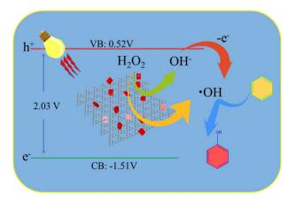
Fig. 7 Schematic diagram of the proposed photocatalytic mechanism.
