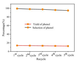
Fig. 5 Regeneration and reusability of g-C<sub>3</sub>N<sub>4</sub>/Zr-Fc MOF. Reaction conditions: catalyst (1.5 mg mL<sup>-1</sup>), benzene (1.6 mL, 18.05 mmol),  $\rm H_2O_2$  (30 wt%) (0.6 mL), acetonitrile (11 mL), trifluoroacetic acid (0.1 g), time: 4 h, and T=333 K.
