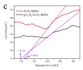
Fig. 4 PL profiles (a) of  $g-C_3N_4$  and  $g-C_3N_4/Zr-Fc$  MOF. Electrochemical impedance profiles (b) and Mott–Schottky diagram (c) of Zr-Fc MOF and  $g-C_3N_4/Zr-Fc$  MOF.
