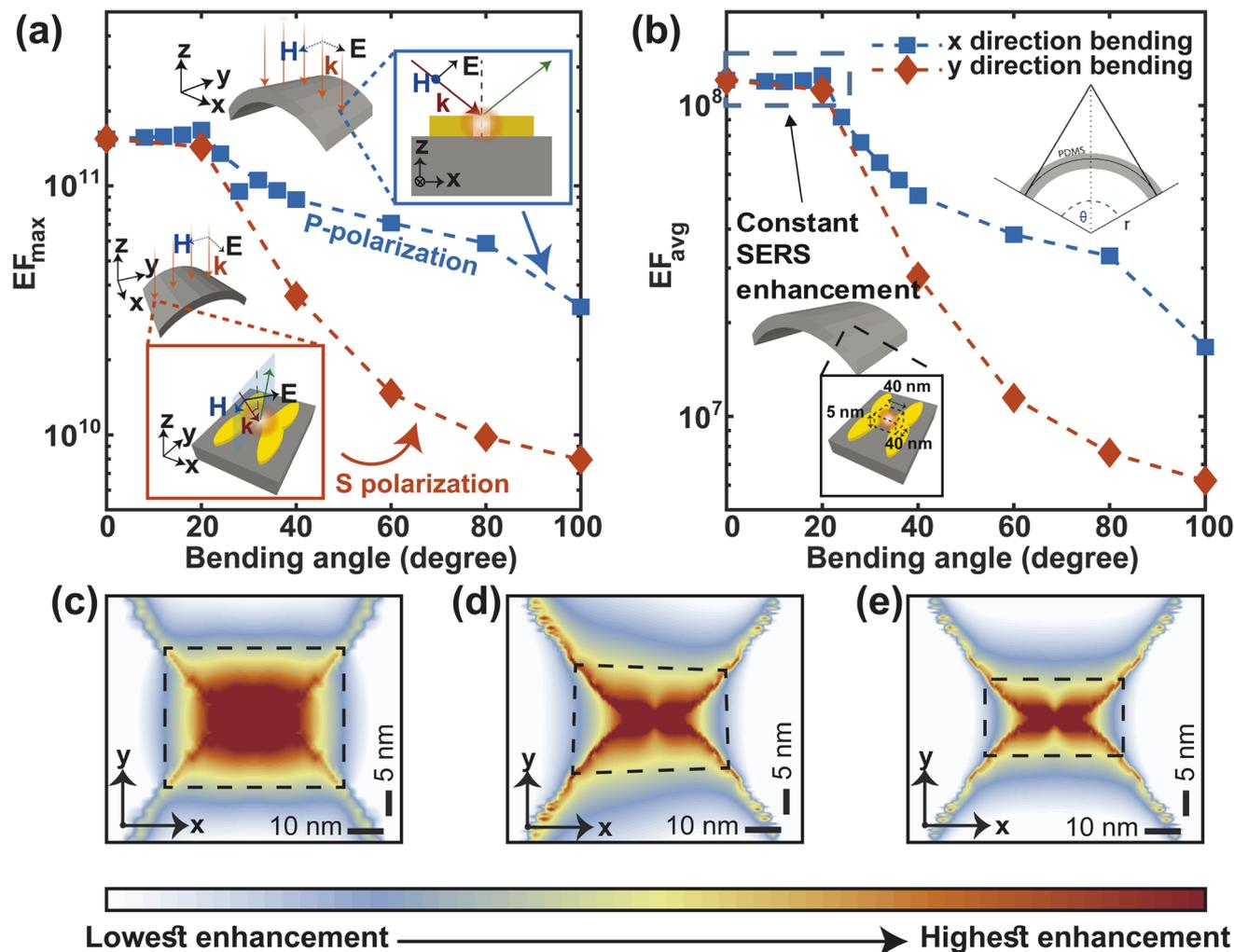
Fig. 8 Changes in SERS enhancement factor,  $EF_{max}$  (a) and  $EF_{avg}$  (b) due to bending. The electric field intensity at the nanogap for three different case, unbent metasurface (c), 100° bending in the x-direction (d) and 100° bending in the y-direction (e).
