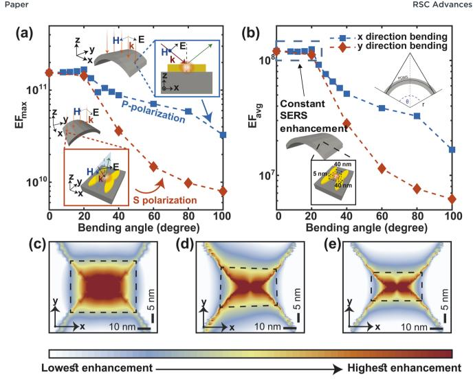
Fig. 8 Changes in SERS enhancement factor,  $EF_{max}$  (a) and  $EF_{avg}$  (b) due to bending. The electric field intensity at the nanogap for three different case, unbent metasurface (c), 100° bending in the x-direction (d) and 100° bending in the y-direction (e).
