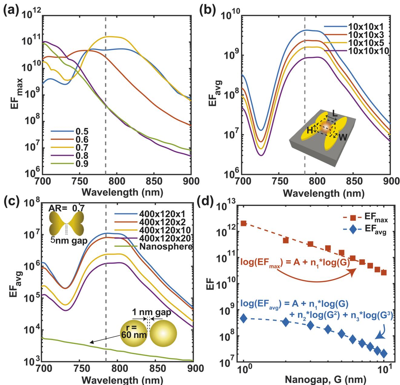
Fig. 6 Maximum EF at different wavelengths for different aspect ratios (a). Average EF over different volumes for 0.7 aspect ratio at a wavelength of 785 nm (b and c). Log–log plots of  $EF_{\max}$  and  $EF_{\text{avg}}$  as a function of nanogap,  $G$  at 785 nm wavelength (d). The fitting parameters are listed in Table 2.
