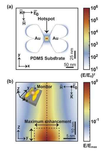
Fig. 7 Profile of electric field intensity at z = 0 (a). Change in maximum EF as vertical distance from the substrate increases (b).
