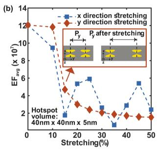
Fig. 9 Changes in SERS enhancement factor,  $\rm EF_{max}$  (a) and  $\rm EF_{avg}(b)$  due to stretching.
