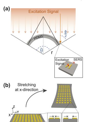
Fig. 3 Modelling of (a) bending (b) stretching to approximate the SERS performance of the proposed metasurface.
