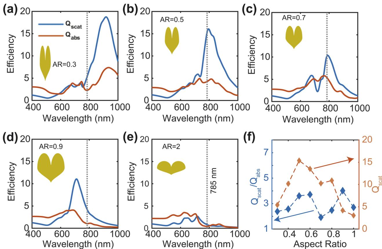
Fig. 4 Scattering and absorption efficiency for different AR (a–e). Scattering to absorption ratio and Scattering efficiency for different AR at 785 nm wavelength (f). The height of the NP is 45 nm.
