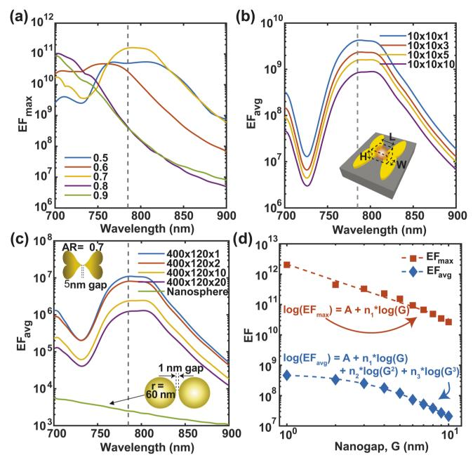
Fig. 6 Maximum EF at different wavelengths for different aspect ratios (a). Average EF over different volumes for 0.7 aspect ratio at a wavelength of 785 nm (b and c). Log-log plots of EF<sub>max</sub> and EF<sub>avg</sub> as a function of nanogap, G at 785 nm wavelength (d). The fitting parameters are listed in Table 2.
