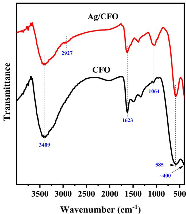
Fig. 5 FT-IR spectra of CFO and Ag/CFO NPs.
