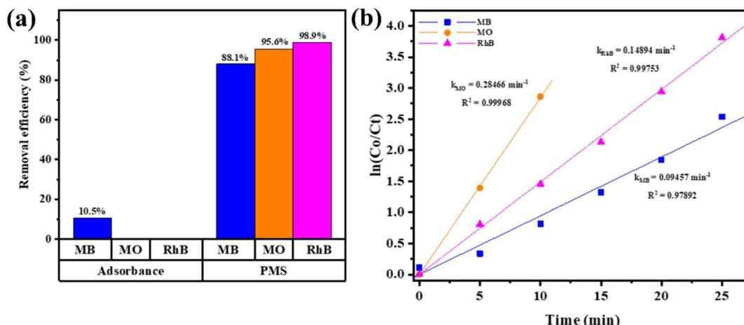
Fig. 10 (a) The removal efficiency of dyes varies in each process after 60 min, and (b) the graph of  $\ln(C_0/C_t)$  vs. time in the Ag/CFO/PMS system.
