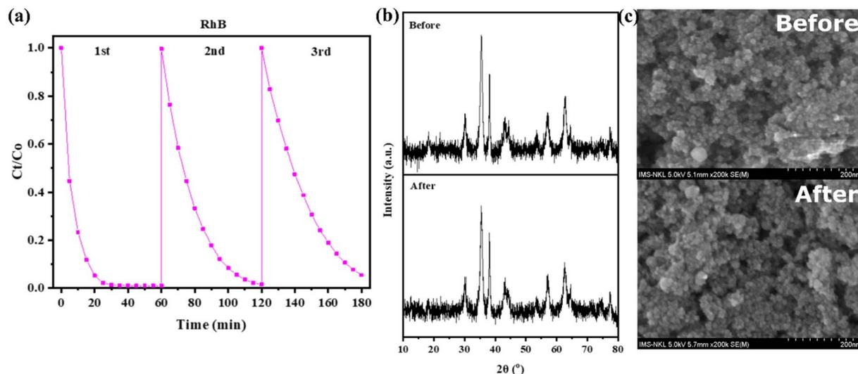
Fig. 13 (a) Reaction efficiency, (b) XRD diagram, and (c) FESEM images of Ag/CFO NPs after three runs.
