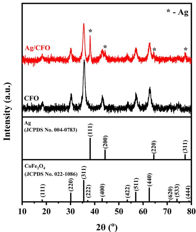
Fig. 3 XRD patterns of CFO and Ag/CFO NPs.
