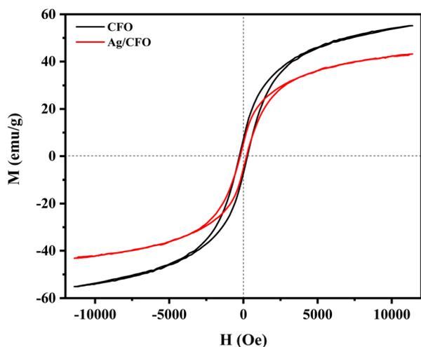
Fig. 12 M–H loops of CFO and Ag/CFO NPs.
