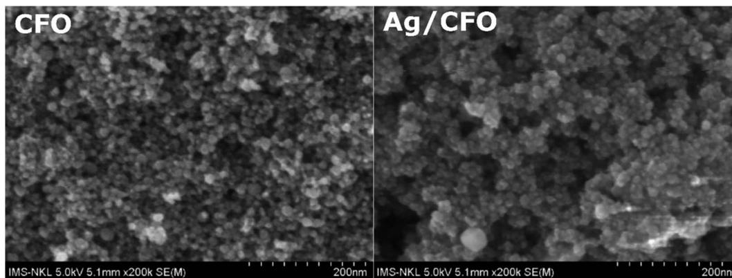
Fig. 6 FE-SEM images of CFO and Ag/CFO NPs.
