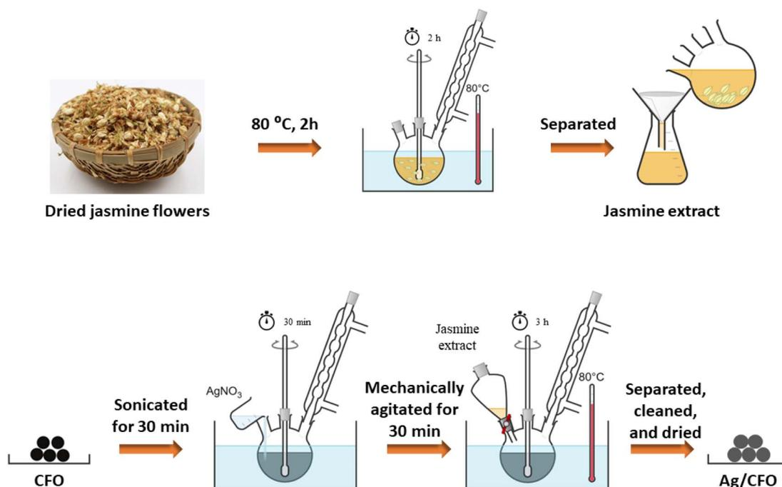
Fig. 2 The synthesis process of Ag/CFO nanoparticles.
