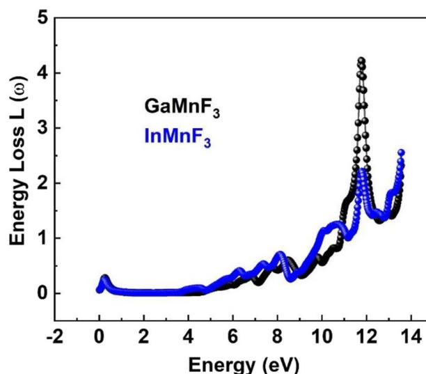
Fig. 13 The energy loss function for ternary QMnF<sub>3</sub> (where Q = Ga, In) fluoroperovskites.
