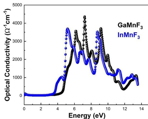
Fig. 10 Optical conductivity of ternary QMnF<sub>3</sub> (where Q = Ga, In) fluoro-perovskites.
