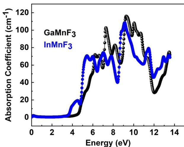
Fig. 8 The absorption coefficient for the QMnF<sub>3</sub> (where Q = Ga, In) fluoro-perovskites.
