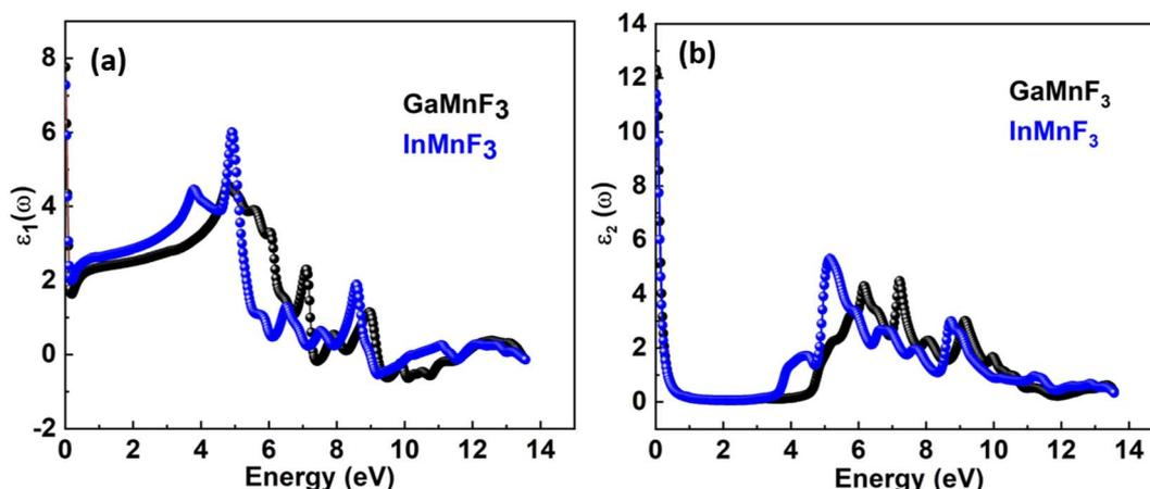
Fig. 7 Real (a) and imaginary (b) parts of the dielectric function of QMnF<sub>3</sub> (where Q = Ga, In) fluoro-perovskites.
