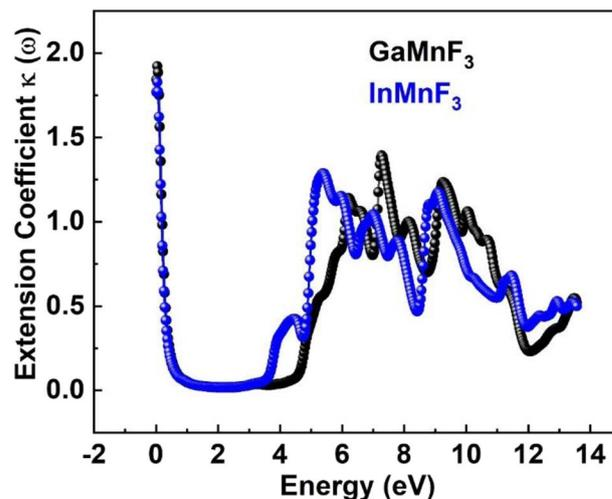
Fig. 12 Extension Coefficient for ternary QMnF<sub>3</sub> (where Q = Ga, In) fluoroperovskites compounds.
