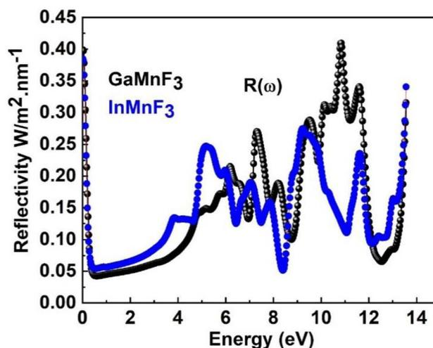
Fig. 9 The reflectivity of the QMnF<sub>3</sub> (where Q = Ga, In) fluoro-perovskites.
