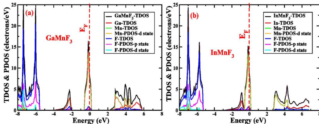
Fig. 6 The total density of states and partial density of states (a) GaMnF<sub>3</sub> (b) InMnF<sub>3</sub> ternary fluoroperovskites compounds.
