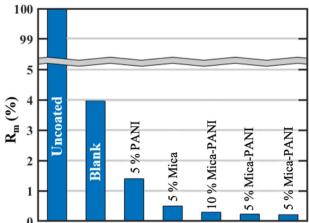
Fig. 12 Graphical representation of percentage of corrosion rate RM% for bare mild steel, blank coating, (16%) PANI coating, (16%) mica coating and composite paint coatings.
