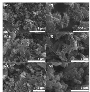
Fig. 3 The two different magnifications of the (a1) and (a2) nano-mica with low-focused and highly-focused images (b1) and (b2) PANI with low-focused and highly-focused images (c1) and (c2) Mica-PANI composite with low focused and highly-focused images.
