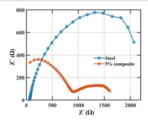
Fig. 9 Nyquist plot for electrochemical impedance data.
