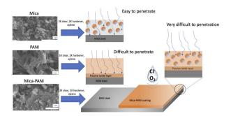
Fig. 1 Schematic representation of the anticorrosive coatings.
