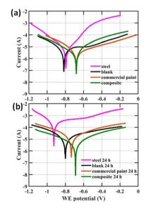
Fig. 7 Tafel plots for comparison of the Mica-PANI composite and commercial paint (a) initial equilibrium (b) 24 h after dipping the coating inside the 0.1 M, 30 mL NaCl solution.
