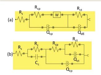
Fig. 8 Equivalent circuit used to obtain electrochemical impedance data.
