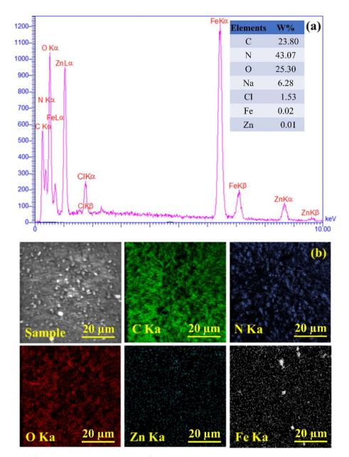
Fig. 2 (a) EDX analysis and (b) element mapping of CN-Pr-Mel/ZnFe $_2O_4$ /CMC hydrogel nanobiocomposites.
