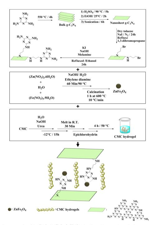
$\textbf{Scheme 1} \quad \textbf{Schematic representation of the CN-Pr-Mel/ZnFe}_2O_4/CMC \ \ \textbf{hydrogel nanobiocomposite synthesis steps}.$
