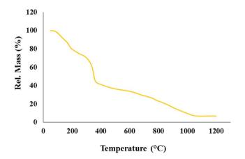
Fig. 5 TGA curve of CN-Pr-Mel/ZnFe $_2$ O $_4$ /CMC hydrogel nanobiocomposite.
