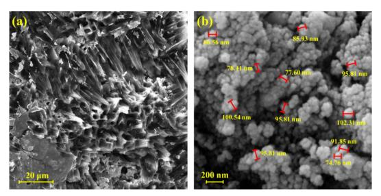
Fig. 3 FE-SEM image of (a) CMC hydrogel and (b) CN-Pr-Mel/ZnFe<sub>2</sub>O<sub>4</sub>/CMC hydrogel nanobiocomposite.
