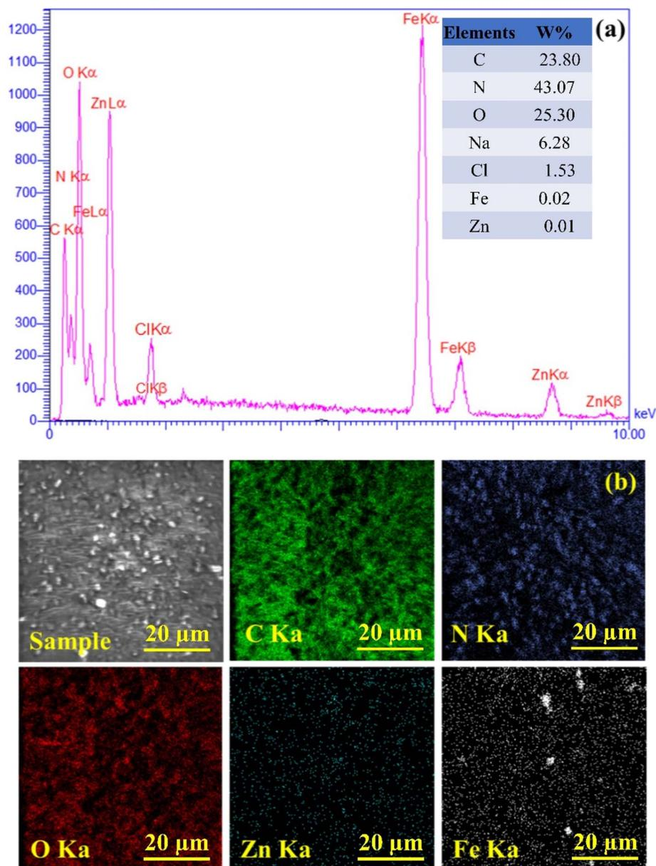
Fig. 2 (a) EDX analysis and (b) element mapping of CN-Pr-Mel/ZnFe<sub>2</sub>O<sub>4</sub>/CMC hydrogel nanobiocomposites.
