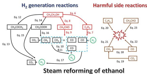
Fig. 2 Main H<sub>2</sub> generation reactions and harmful side reactions in SRE.
