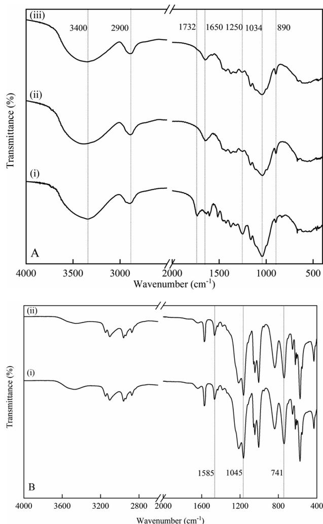
Fig. 3 (A) Normalized FTIR spectrum of (i) CC, (ii) ACC, and (iii) IL-CCCNC. (B) Normalized FTIR spectrum of (i) pure [Bmim][HSO<sub>4</sub>] and (ii) regenerated [Bmim][HSO<sub>4</sub>].
