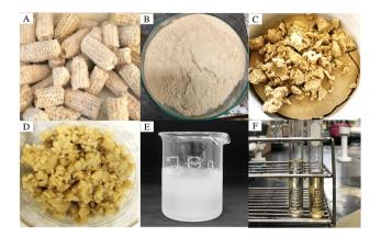
Fig. 1 (A) Corncob, (B) ground and sieved sample, (C) water-soaked sample, (D) alkaline-pretreated sample, (E) [Bmim][HSO<sub>4</sub>] hydrolyzed corncob, (F) fresh (left) and regenerated (right) [Bmim][HSO<sub>4</sub>].
