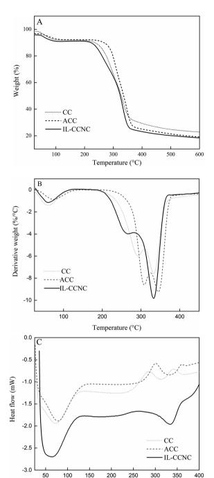
Fig. 7 (A) TGA curves of CC, ACC and IL-CCCNC. (B) DTG curves of CC, ACC and IL-CCCNC. (C) DSC curves of CC, ACC and IL-CCCNC.
