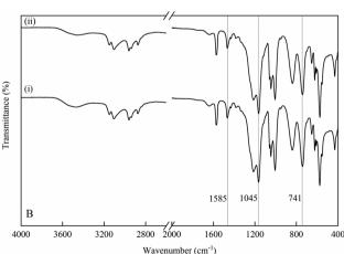
Fig. 3 (A) Normalized FTIR spectrum of (i) CC, (ii) ACC, and (iii) IL-CCCNC. (B) Normalized FTIR spectrum of (i) pure [Bmim][HSO<sub>4</sub>] and (ii) regenerated [Bmim][HSO<sub>4</sub>].
