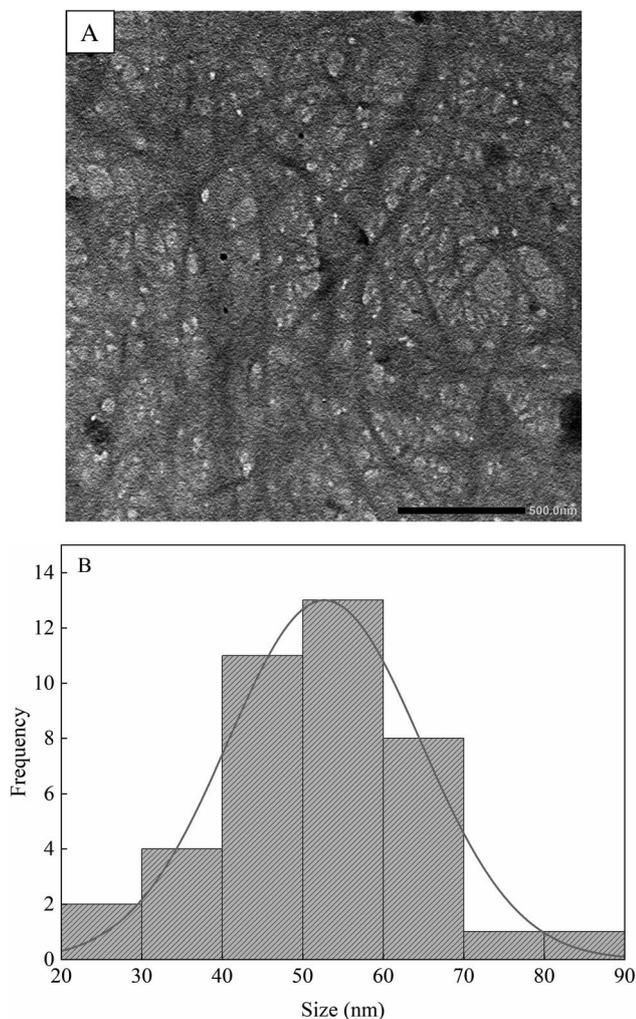
Fig. 6 (A) TEM image of IL-CCCNC; (B) diameter size distribution of IL-CCCNC.
