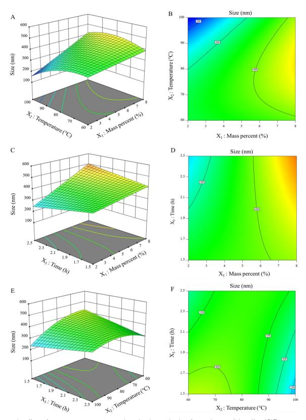
Fig. 2 Interactive effects of mass percent, temperature, and reaction time on the size of corncob nanocellulose. (A and B) Temperature vs. mass percent at reaction time of 2 h; (C and D) time vs. mass percent at reaction temperature of 80 °C; (E and F) time vs. temperature at mass percent of 5%.
