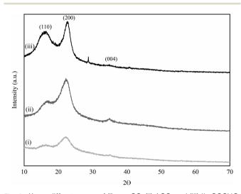
Fig. 4 X-ray diffractogram of (i) raw CC, (ii) ACC, and (iii) IL-CCCNC.
