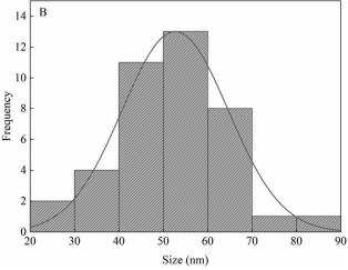
Fig. 6 (A) TEM image of IL-CCCNC; (B) diameter size distribution of IL-CCCNC.
