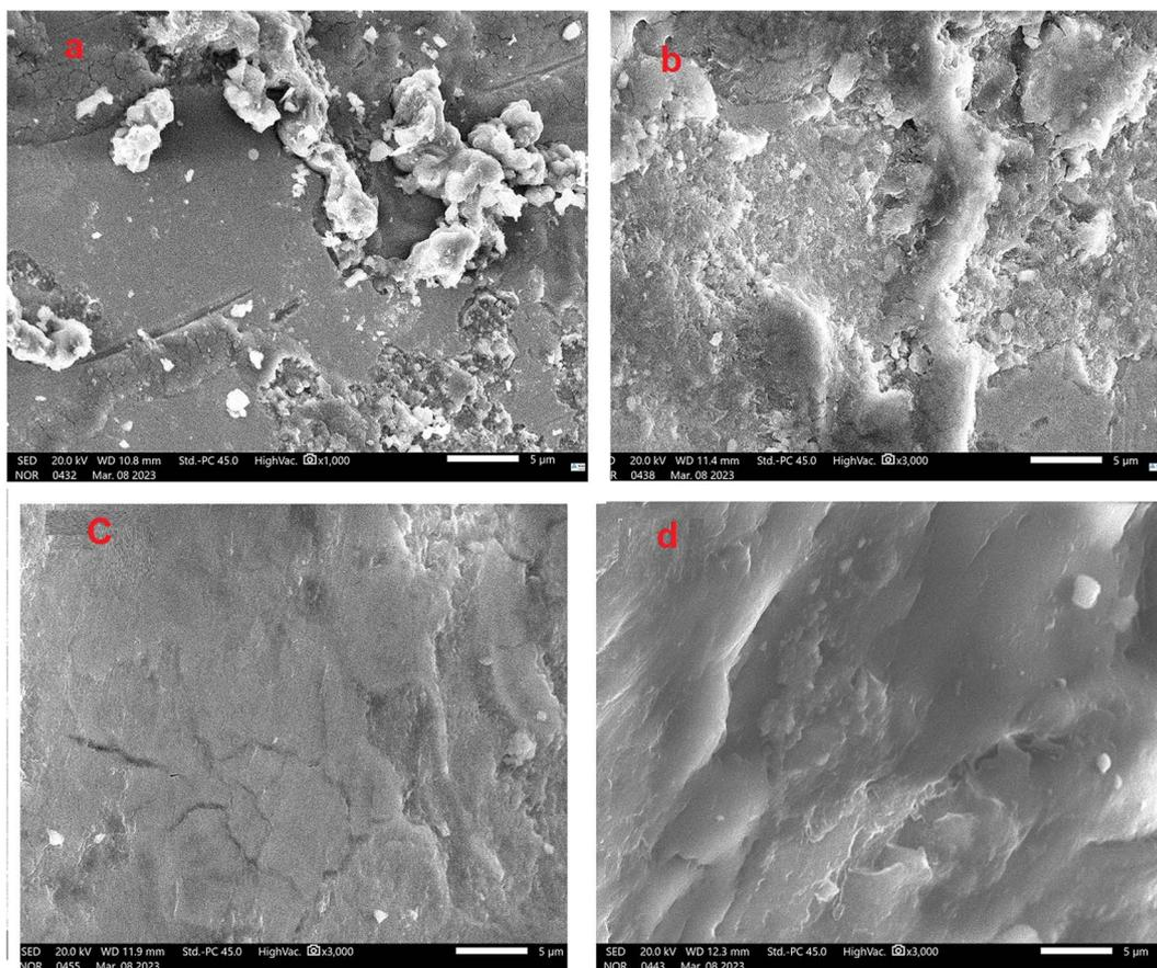
Fig. 7 FESEM images of the worn ball during the EP test with (a) commercial oil, (b) commercial oil with 20% PE ester, (c) 0.05% graphene dispersed commercial oil with 20% PE ester, and (d) 0.05% graphene dispersed commercial oil with 30% PE ester.
