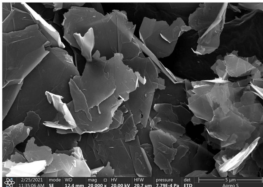
Fig. 1 FESEM image of graphene nanoplatelets.
