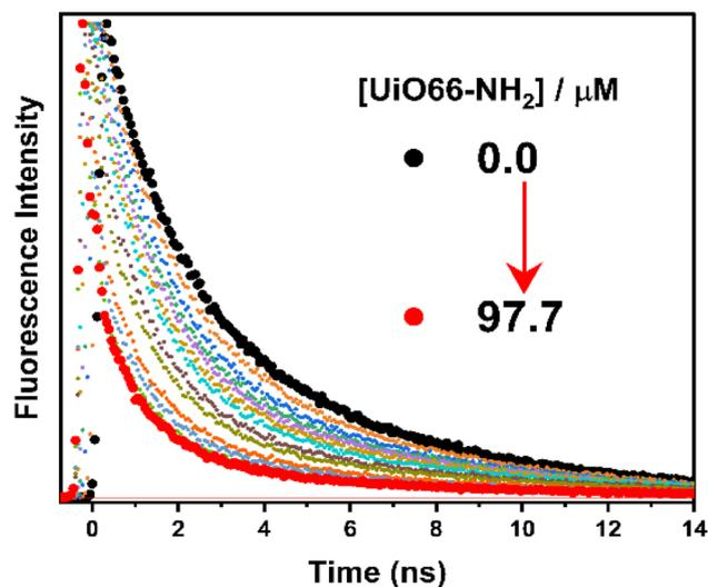
Fig. 7 TCSPC decay profiles for titration of H<sub>2</sub>TMPyP (3.0  $\mu\text{M}$ ) with UiO-66 (0–97.7  $\mu\text{M}$ ). The excitation light was fixed at 439 nm.
