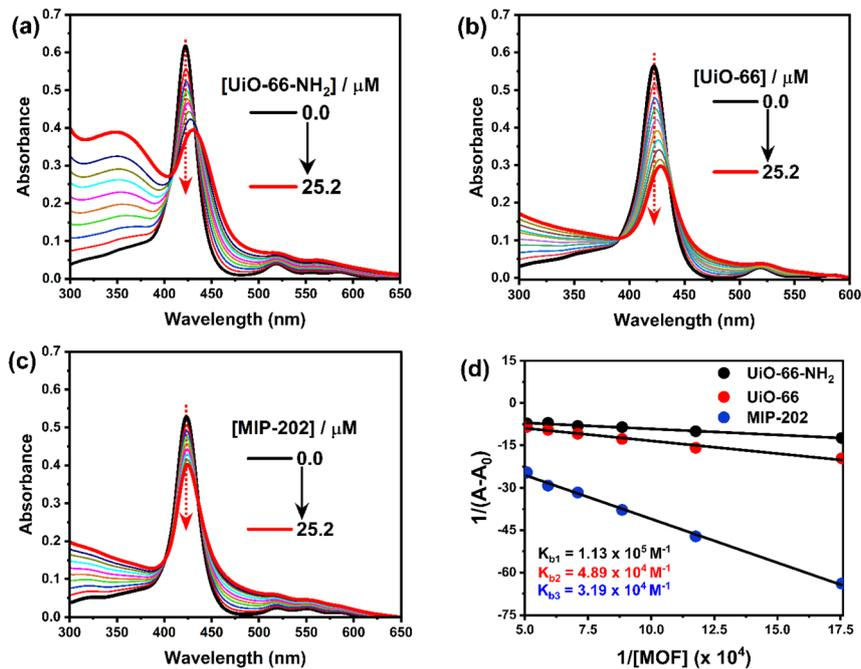
Fig. 5 UV-vis absorption spectra of photometric titration of  $\text{H}_2\text{TMPyP}$  ( $3.0 \mu\text{M}$ ) in the presence of: (a) UiO-66, (b) UiO-66-NH<sub>2</sub>, (c) MIP-202, (d) Benesi-Hildebrand plot for the three titrations to determine the binding constant  $K_b$ .
