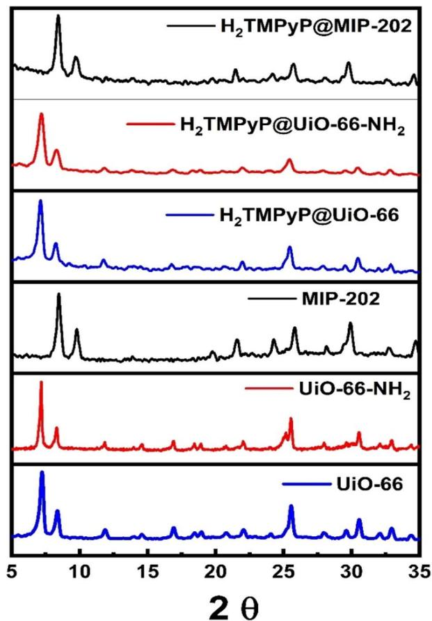
Fig. 1 XRD of the synthesized UiO-66, UiO-66-NH<sub>2</sub>, and MIP-202.
