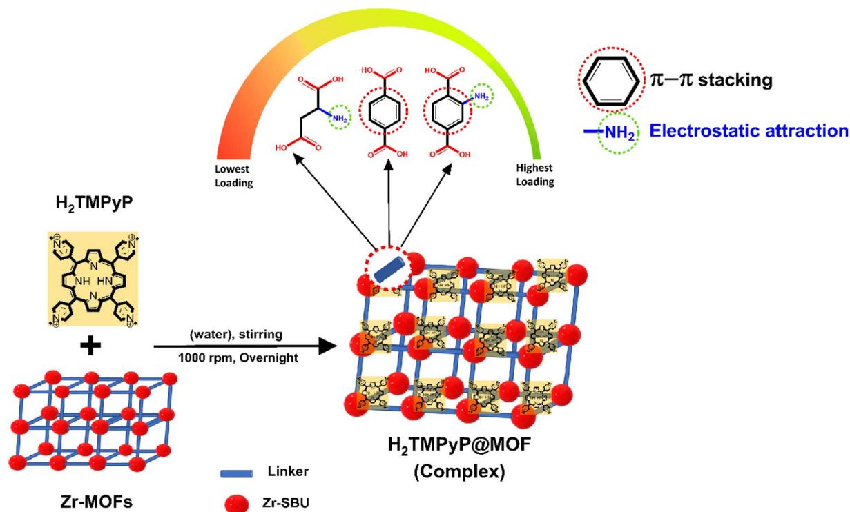
Scheme 1 Schematic representation of the building blocks of the three MOFs and their targeted non-covalent interactions with H<sub>2</sub>TMPyP.
