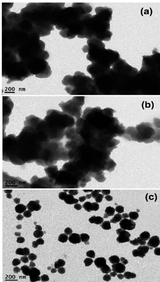
Fig. 2 HR-TEM images of (a)  $\text{H}_2\text{TMPyP}@ \text{UiO}-66-\text{NH}_2$  complex, (b)  $\text{H}_2\text{TMPyP}@ \text{UiO}-66$  complex, and (c)  $\text{H}_2\text{TMPyP}@ \text{MIP}-202$  complex.
