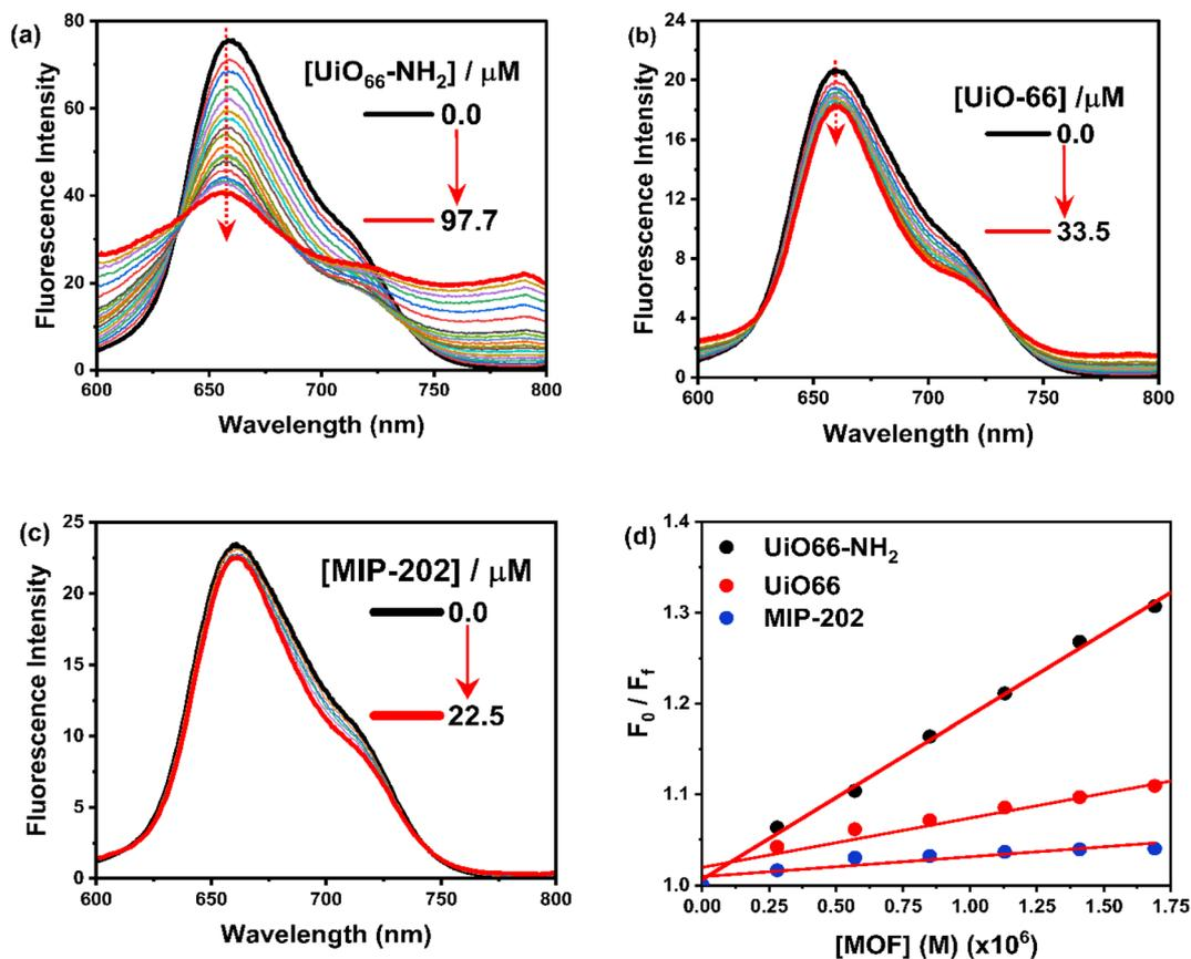
Fig. 6 Fluorescence spectra for titration of  $\text{H}_2\text{TMPyP}$  ( $3.0 \mu\text{M}$ ) of  $\text{H}_2\text{TMPyP}$  ( $3.0 \mu\text{M}$ ) in the presence of (a) UiO-66, (b) UiO-66-NH<sub>2</sub>, (c) MIP-202. The concentrations of MOFs were kept at (0–25.2  $\mu\text{M}$ ). (d) Stern-Volmer plots.
