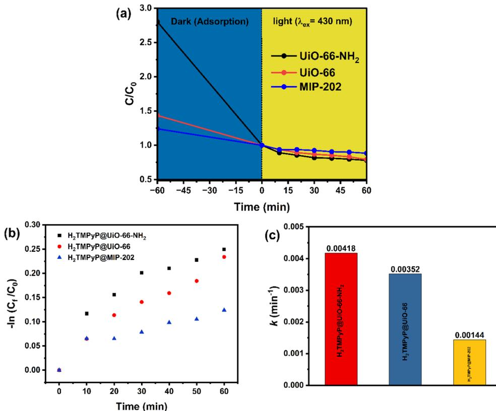
Fig. 9 (a) Rate of photodegradation of MO dye under ( $\lambda_{\text{ex}} = 430 \text{ nm}$ ) light irradiation [conditions: catalyst dosage of 10 mg, MB concentration of  $20 \text{ mg L}^{-1}$ ], (b) first-order reaction kinetics of the photocatalytic degradation of MO using H<sub>2</sub>TMPyP@MOF composites, and (c) rate constant values ( $k$ ) of the photocatalytic degradation reaction of MO using H<sub>2</sub>TMPyP@MOF composites.
