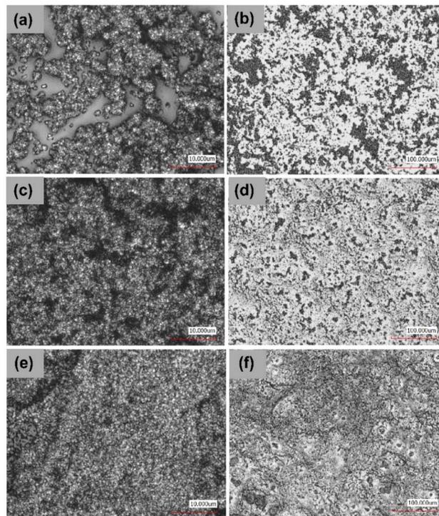
Fig. 8 Laser scanning confocal microscope images of: (a) UiO-66-NH<sub>2</sub>, (b) H<sub>2</sub>TMPyP@UiO-66-NH<sub>2</sub> complex, (c) UiO-66, (d) H<sub>2</sub>TMPyP@UiO-66 complex, (e) MIP-202, and (f) H<sub>2</sub>TMPyP@MIP-202 complex.
