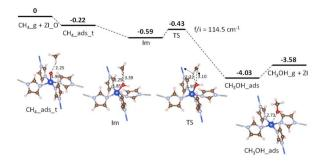
Fig. 6 Potential energy surface for  $CH_4$  conversion over  $ZI_-O$  via the  $CH_4$ —ads\_t pathway. Relative energies are given in eV. The zero-reference energy is the sum of the total energies of the isolated  $CH_4$  molecule and  $ZI_-O$ . Zero-point energy correction is not included.
