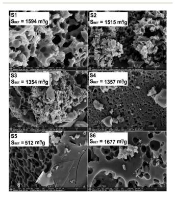
Fig. 1 SEM micrographs and the specific surface area (from BET analysis) for the porous carbon-based samples. Note, the scale bars at the bottom right of the SE micrographs are  $4 \mu m$ .
