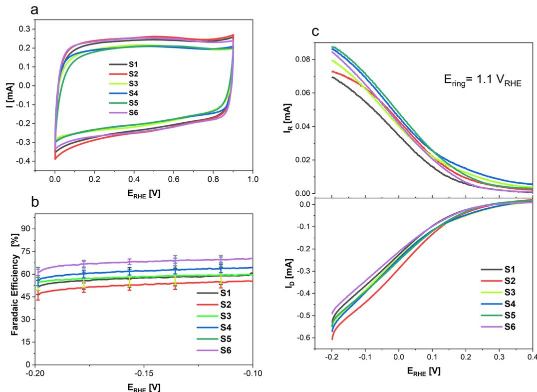
Fig. 6 Linear sweep voltammograms in 0.1 M HClO<sub>4</sub> at 10 mV s<sup>-1</sup> and 1600 rpm where (a) shows cyclic voltammograms in Ar-saturated 0.1 M HClO<sub>4</sub> from 0 to 0.9 V before ORR, (b) shows the FE as a function of electrode potential in O<sub>2</sub>-saturated 0.1 M HClO<sub>4</sub> and (c) shows the ring and disk currents in O<sub>2</sub>-saturated 0.1 M HClO<sub>4</sub>.
