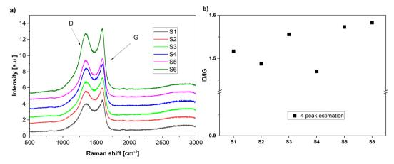
Fig. 3 (a) Raman spectra of the various carbons obtained in the present work. (b) The calculated  $I_D/I_G$  ratios by 4 peak fitting.
