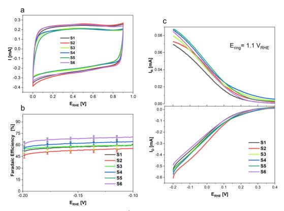
Fig. 6 Linear sweep voltammograms in 0.1 M HClO $_4$  at 10 mV s $^{-1}$  and 1600 rpm where (a) shows cyclic voltammograms in Ar-saturated 0.1 M HClO $_4$  from 0 to 0.9 V before ORR, (b) shows the FE as a function of electrode potential in  $O_2$ -saturated 0.1 M HClO $_4$  and (c) shows the ring and disk currents in  $O_2$ -saturated 0.1 M HClO $_4$ .
