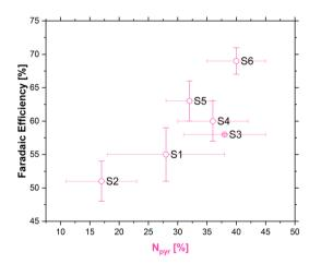
Fig. 7 Correlation between pyridinic nitrogen content (from XPS) and FE [%].
